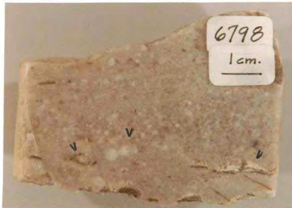
FIG. 25d— Poorly-cemented patches over pebbles and clay clasts (arrows). Depth in feet.
