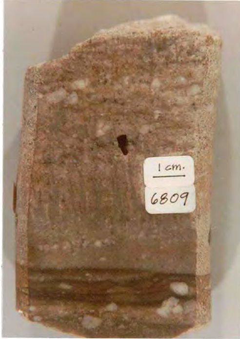
FIG. 25c— Irregular lower digitate boundary, similar to the lower boundaries in poorly cemented disk-shaped lenses found in outcrop. Depth in feet.
