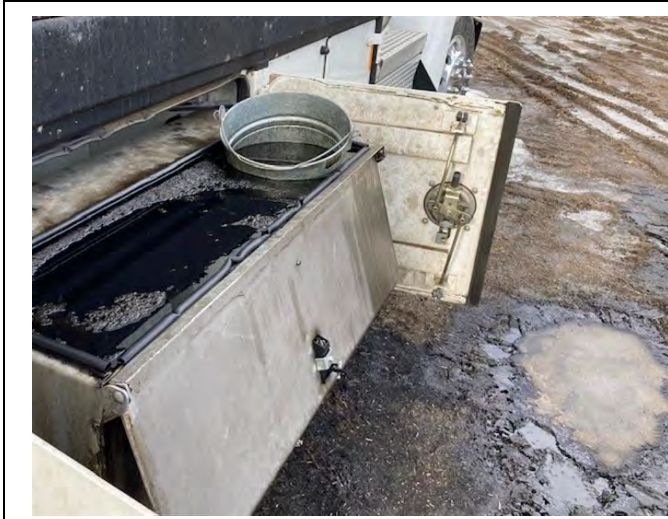
Laydown Yard – MVP-LY-068 – A leak occurred from a service truck that stored used engine oil. About 3 gallons of the used engine oil spilled. The crew contained the spill immediately and began cleaning it up (December 30, 2020) – MP 0.0 – Communication
