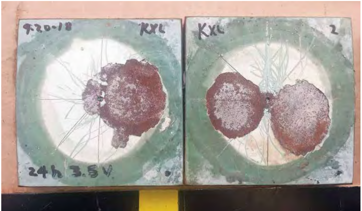
Figure 5. Cathodic disbondment test results for the non-whitewashed pipe ends exposed to ultraviolet.
