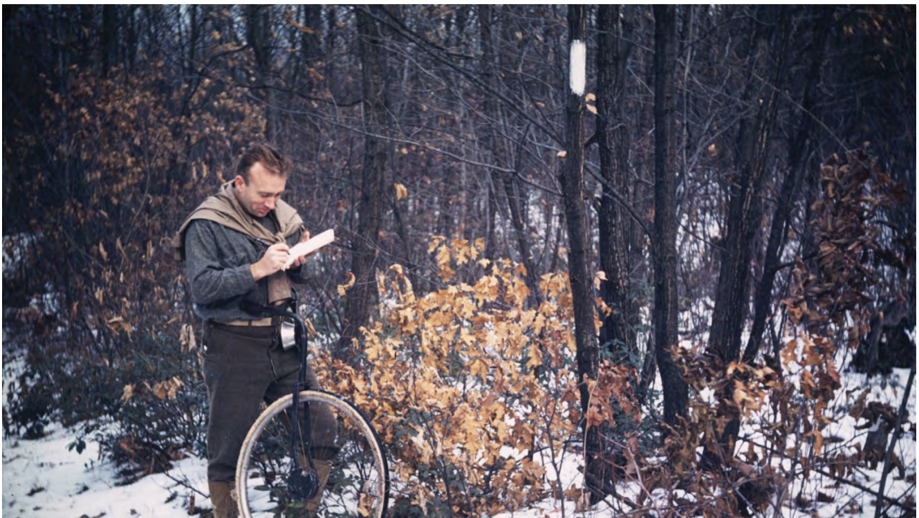
Myron Avery is pictured here with one of his constant companions: a measuring wheel used to tally the length of the A.T.
