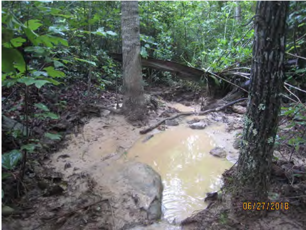
Photo 1: Sedimentation within "SMM-15" ~160' downstream of LOD; Depth = 3"
