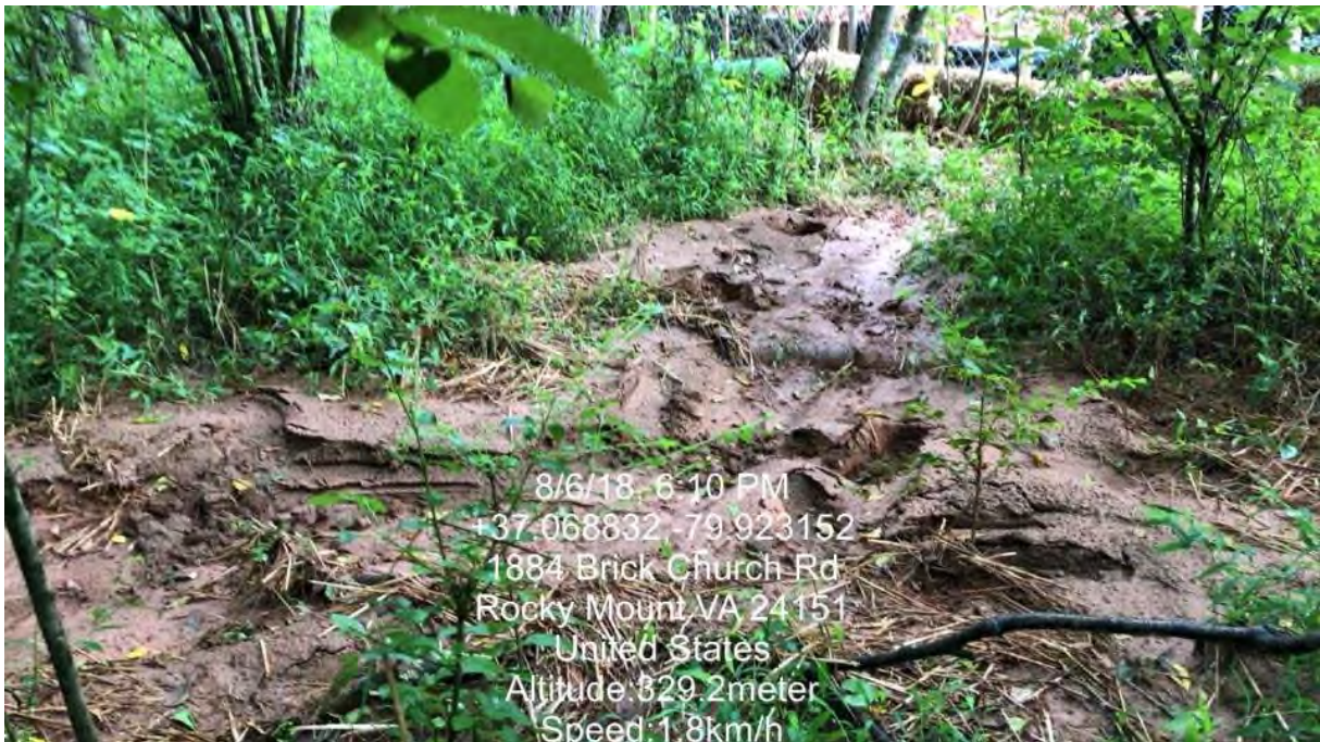
Figure 40 - Sediment deposits off ROW, at UT to Teels Creek, September 23, 2018, Source: citizen monitor
