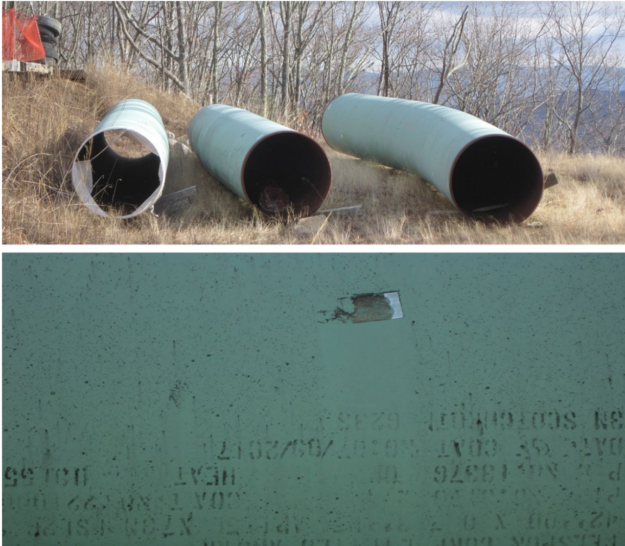
Figure 22. (Above) Pipes stored adjacent to and southeast of the Forest Service’s Brush Mountain Road within the JNF in Montgomery County. (Below) A side view of one of the pipes as is visible from the road. The date “09/2017,” inverted, appears as faded lettering near the center of the photo. A damaged section of the pipe’s exterior is visible above the date, near the top of the photo. Most of the lettering on the pipe is barely visible, a likely result of coating degradation – even though the pigment applied as lettering likely provided some level of protection to the FBE coating immediately beneath it.
