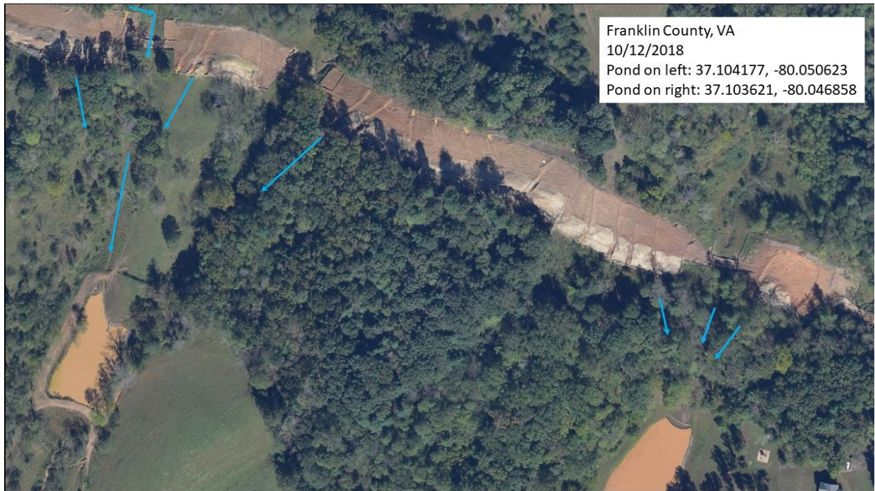
Figure 14: Same location as figures 6 & 7. Sediment laden ponds and flow pattern arrows from MVP construction LOD indicate potential source.
