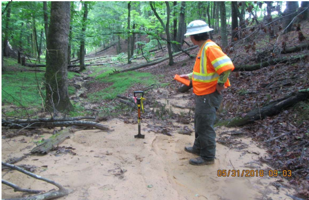
Sediment within channel at debris dam ~420-feet from MVP LOD Depth 3 to 8-inches (average), Maximum depth of 11-inches; Sediment deposit 12-feet wide
