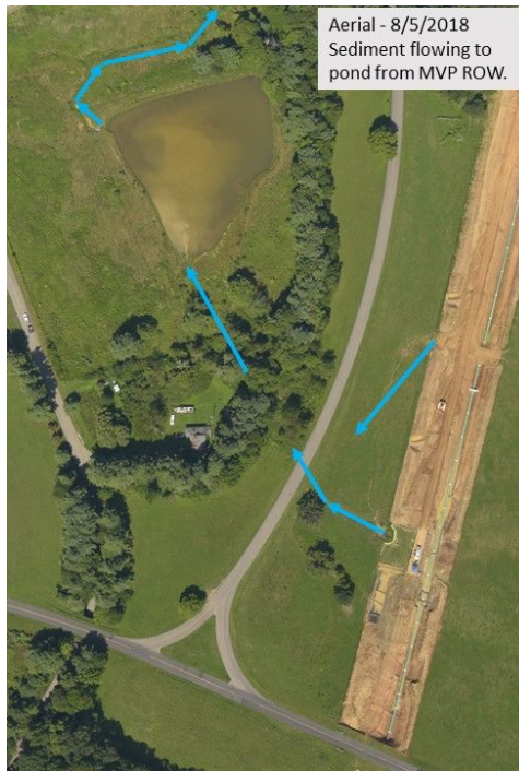
Figure 21: Aerial image from 8/5/2018 (left) and a pre-construction aerial (right) show drainage and sediment impacts from MVP construction ROW to neighboring pond.
