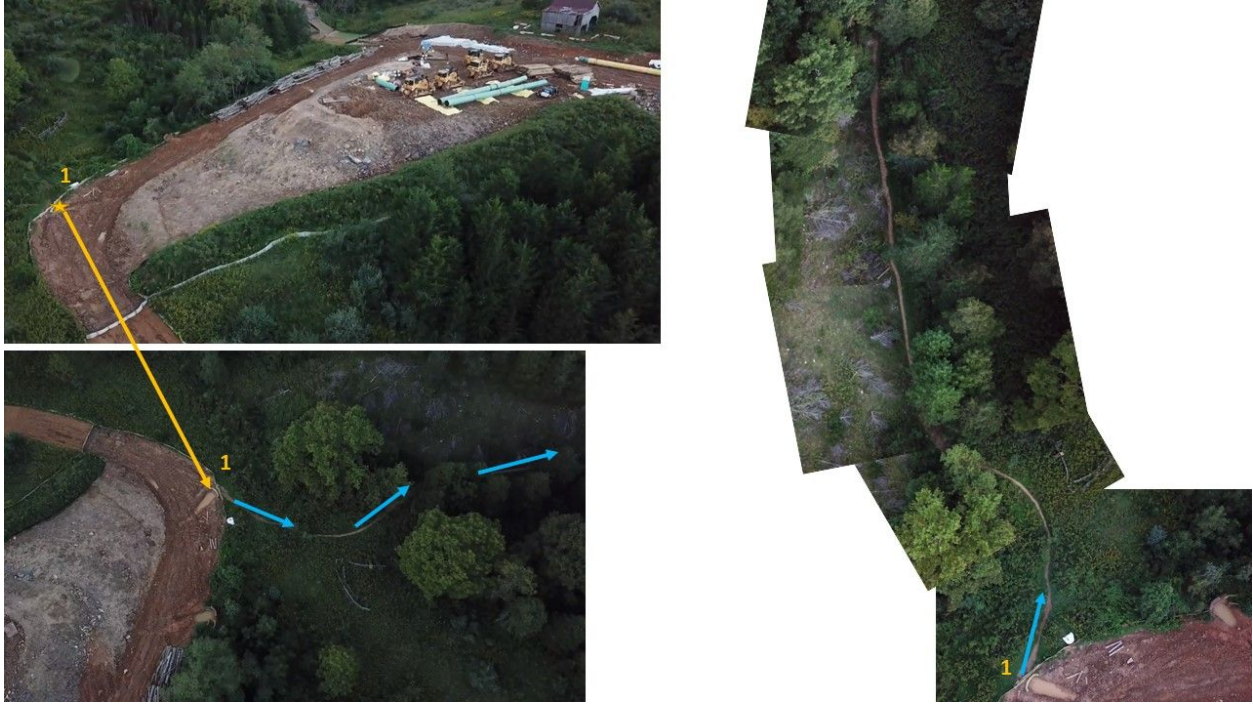
Figure 10: Location 1 shows full catch basins and sediment laden stormwater flowing to the North Fork of the Roanoke River. Flows are constant during every rain event.
