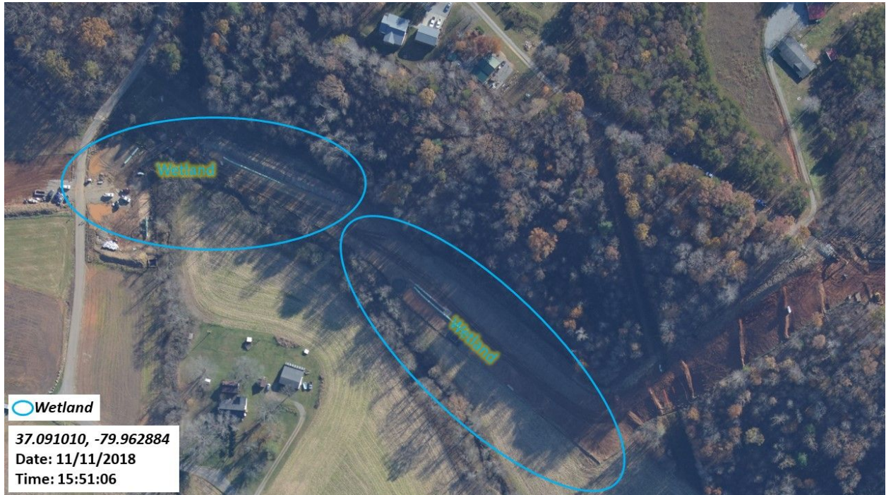
Figure 34: Wetlands area encroachment. Sediment flowing into stream adjacent to right of way.
