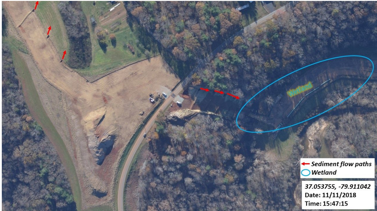
Figure 24: Iron Ridge Road shows discoloration from mud in roadway. Flow paths and wetland identified.
