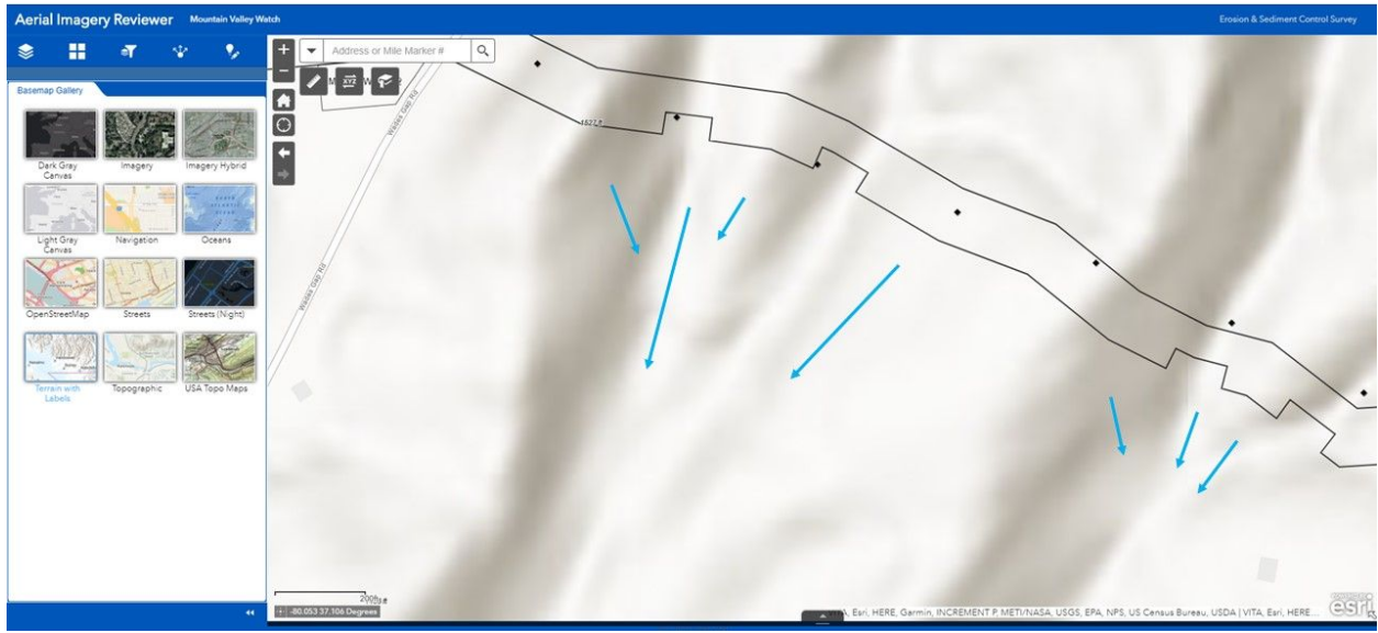
Figure 13: Same location as figure 6, shaded relief map used as basemap showing drainage flow patterns.
