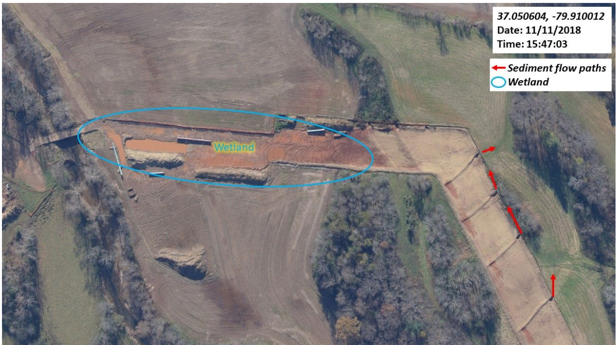
Figure 23: Sediment flowing from waterbars off of pipeline corridor. Sediment ponding in delineated wetlands.
