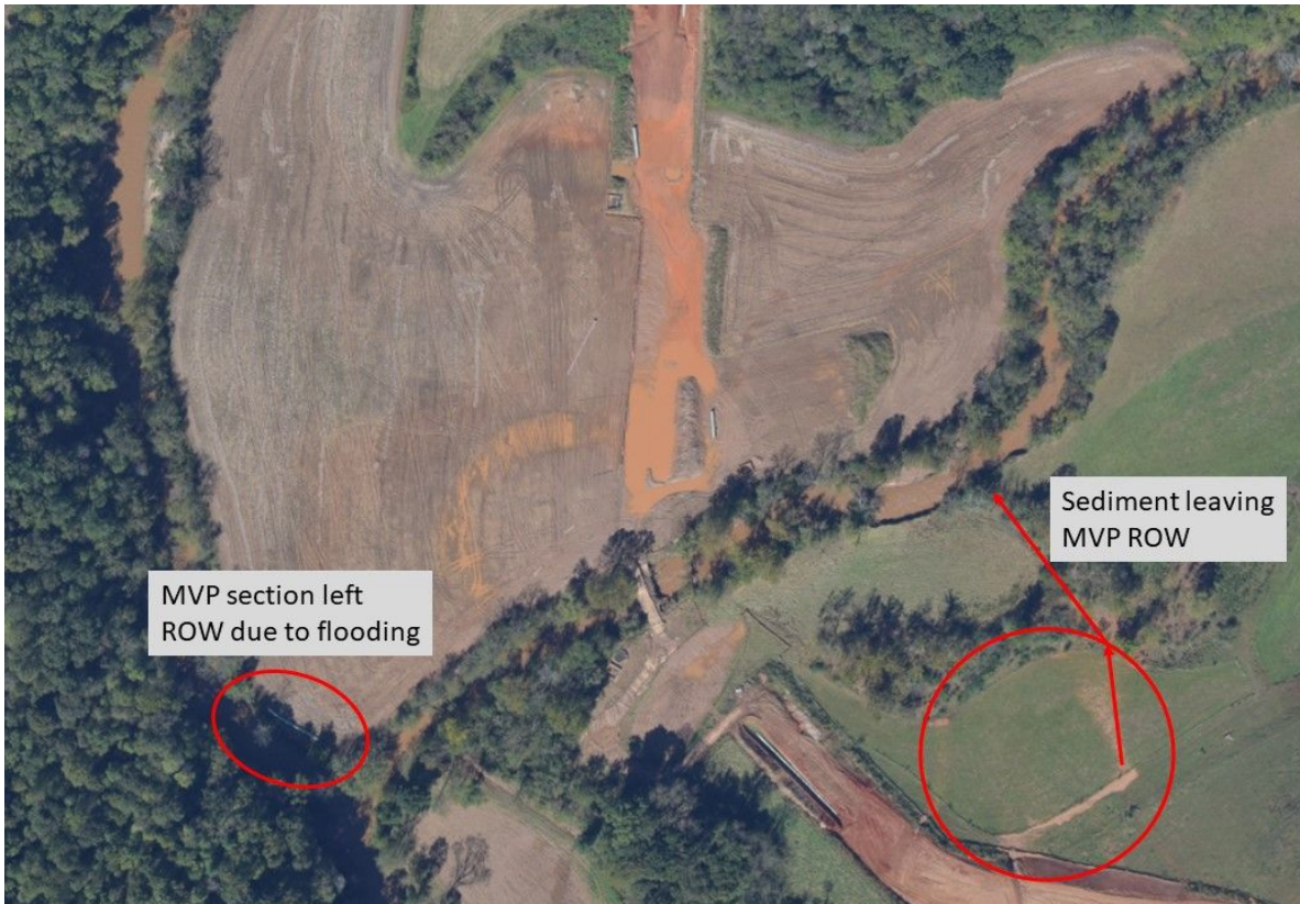
Figure 15: Franklin County, Virginia image (10/12/2018) showing a large section of pipe washed from MVP construction ROW due to flooding.
