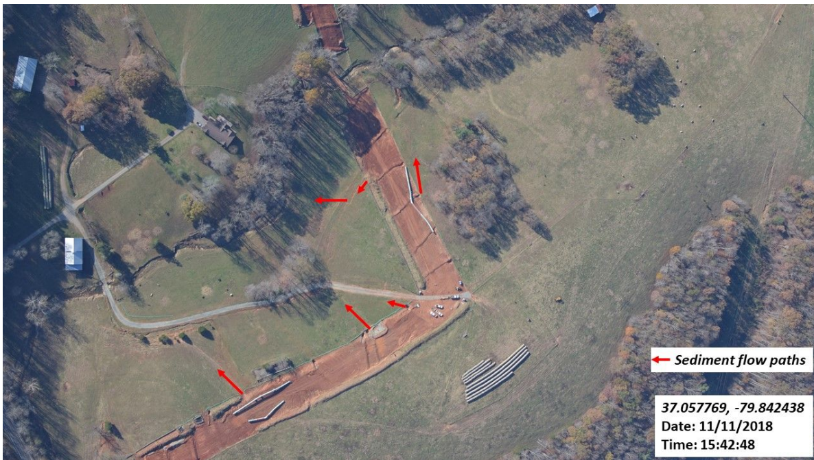
Figure 17: Flow paths where sediment leaves the MVP construction ROW during rain events.
