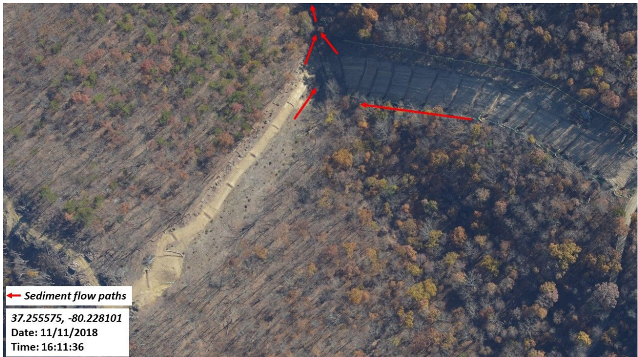
Figure 35: Sediment flowing into stream channel from pipeline right of way. Stream channel is at bottom or slopes.
