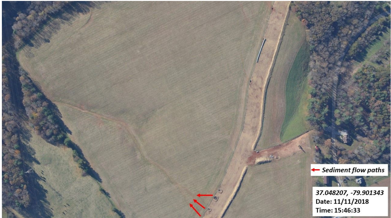
Figure 20: Sediment flowing into adjacent field into drainage channel conveying sediment to stream.
