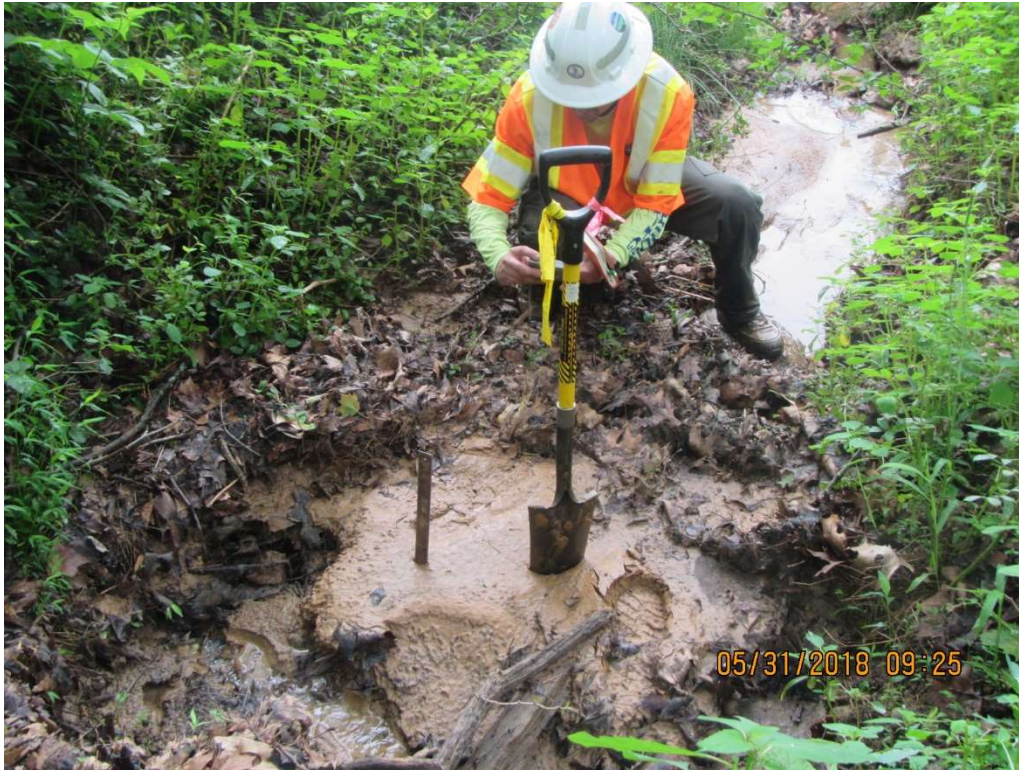
Sediment in channel near treeline ~1,000-feet from MVP LOD Channel 3-feet wide; Sediment depth 6.5-inches
