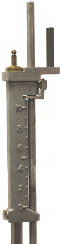
Figure 46. Closeup view of setting scale on handle of top-setting wading rod.
