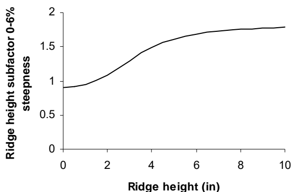
Figure 9.11. Ridge subfactor values as a function of ridge height for land slopes less
