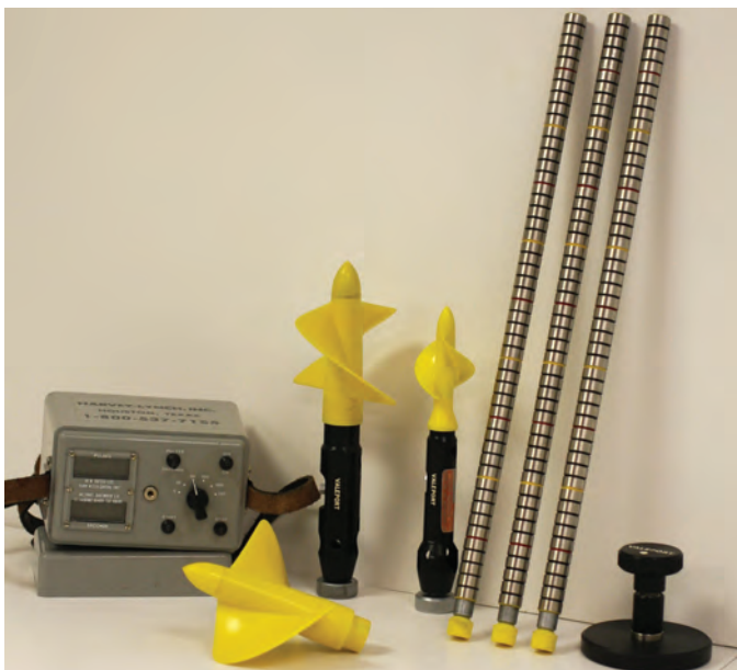
Figure 31. Valeport current meter.
