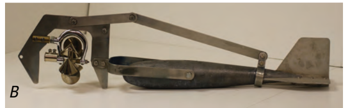
Figure 22. Collapsible hanger assembly for used with 30- and 50-pound C-type weights, for measurements under ice (A, in measurement position and B, collapsed).
