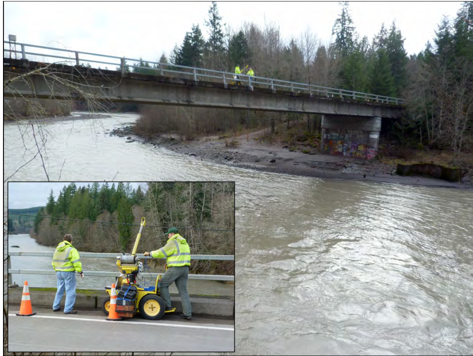
Figure 3. Photographs showing suspended-sediment sampling at Toutle River at Tower Road near Silver Lake, Washington, December 13, 2012. Photographs taken by Kurt Spicer, USGS, Cascades Volcano Observatory.
