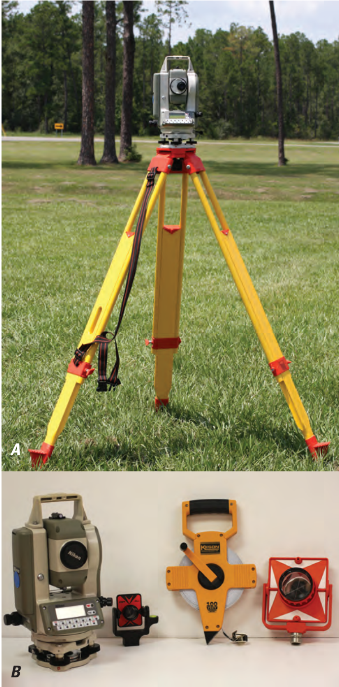
Figure 8. Total station surveying equipment: A, instrument and tripod and B, instrument reflector targets and surveying tape.
