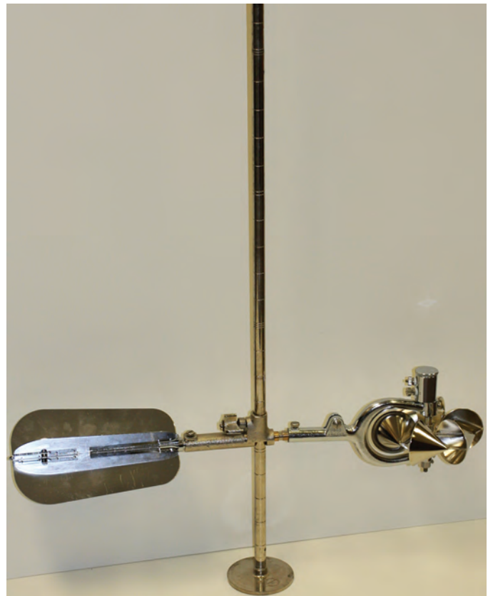
Figure 48. Round wading rod with Price AA current meter attached.
