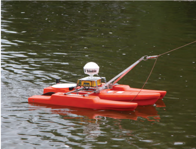
Figure 71. Measuring with a tethered ADCP, DGPS, and trimaran.
