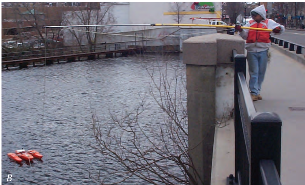
Figure 73. ADCP equipment mounted and operated on A , a moving boat and B , a tethered platform.
