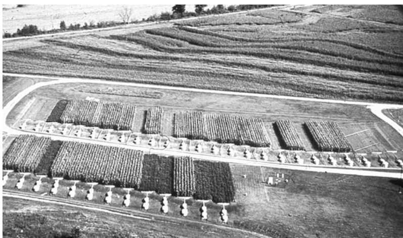
Figure 5.6. Erosion plots 12 ft wide (3.65 m) and 72.6 ft (22.1 m) long near Columbia, MO.
