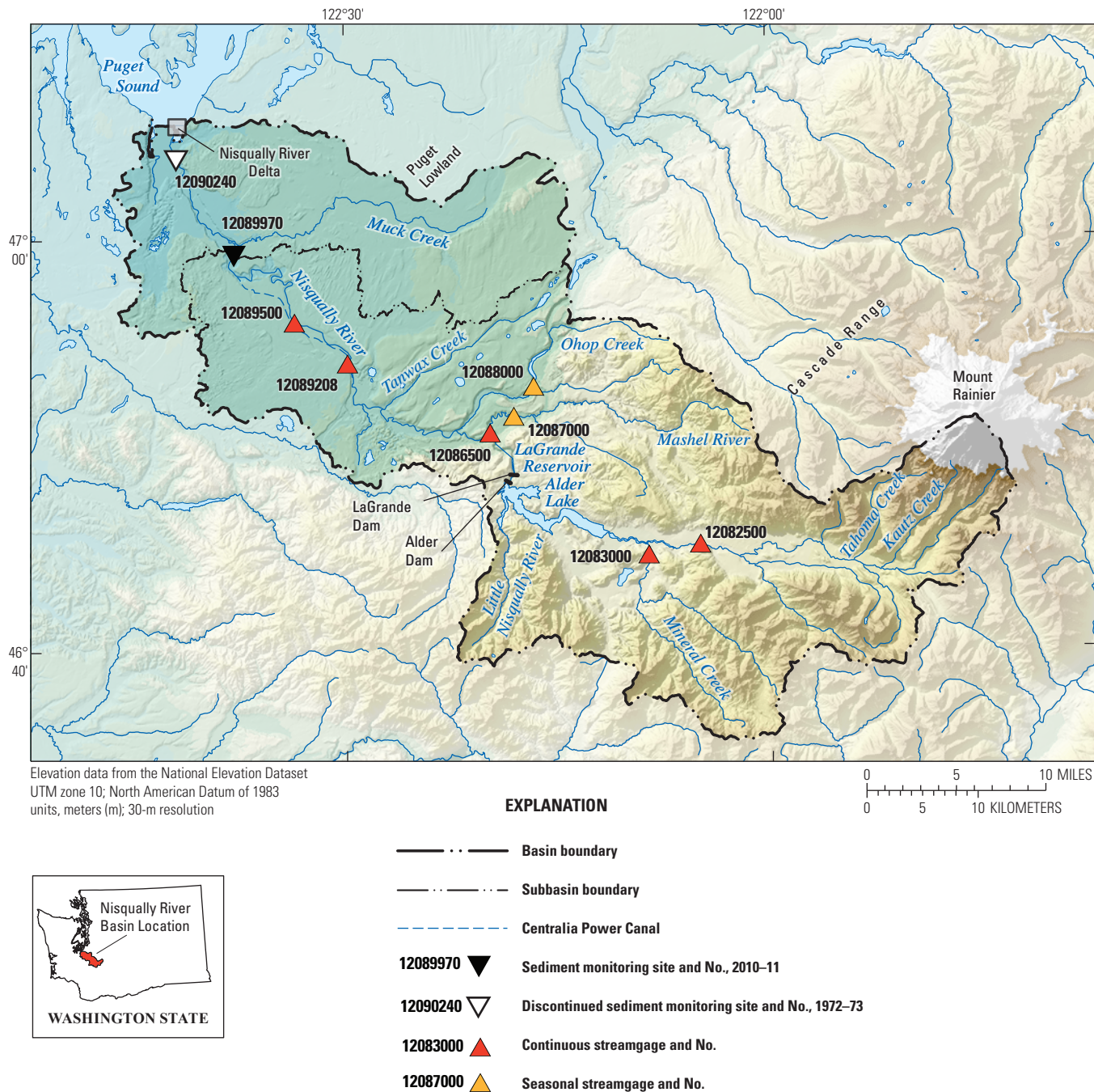
Figure 1. U.S. Geological Survey streamgages and sediment-monitoring site in the Nisqually River Basin, western Washington.
