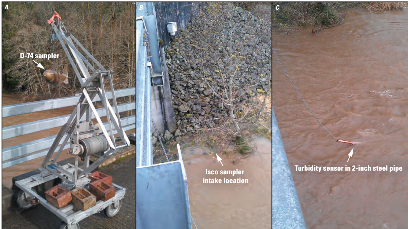
Figure 2. Sediment sampling equipment (A), sample intake area at edge of active channel (B), and turbidity-monitoring installation (C), at the U.S. Geological Survey sediment-monitoring site Nisqually River near Yelm (12089970), Nisqually River Basin, western Washington, March 10, 2011. Photographs by Christopher A. Curran, U.S. Geological Survey.
