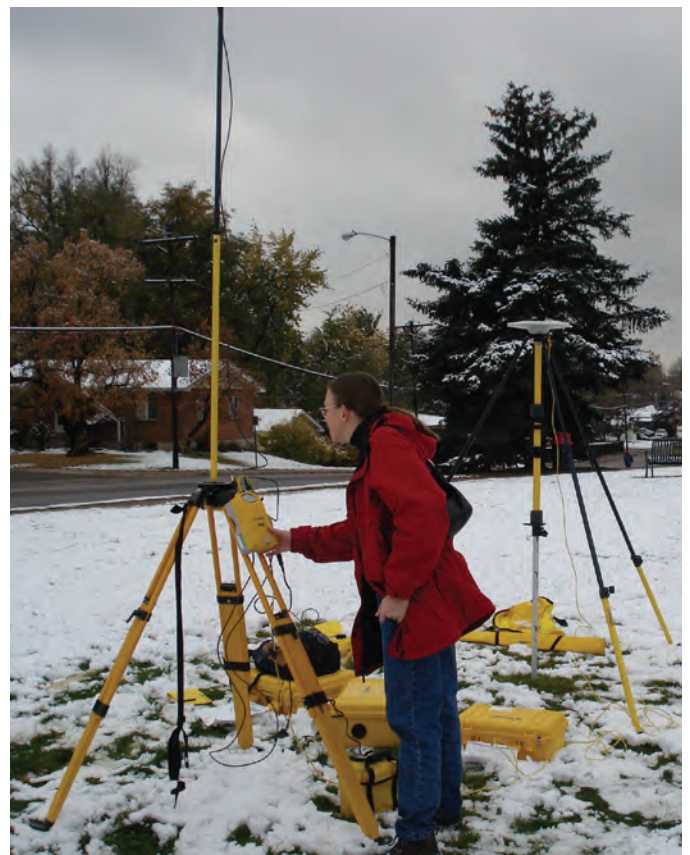
Figure 9. Global positioning system with real-time kinematic (RTK-GPS) base station and radio transmitter.
