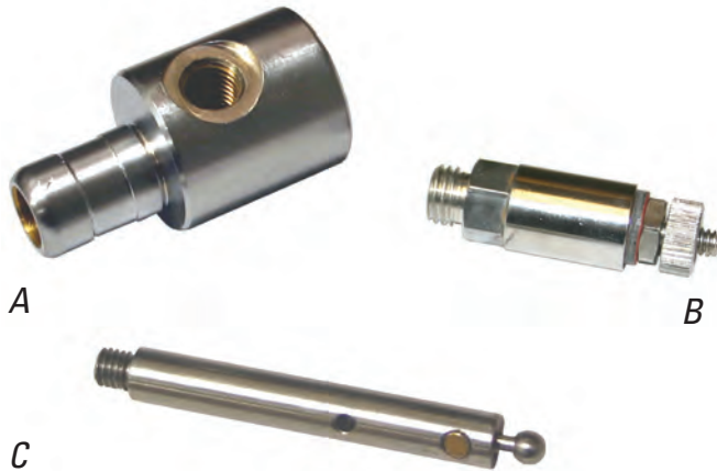
Figure 32. A, Price AA magnetic head current meter contact chamber; B, single count binding post; and C, shaft with magnet for magnetic heads.
