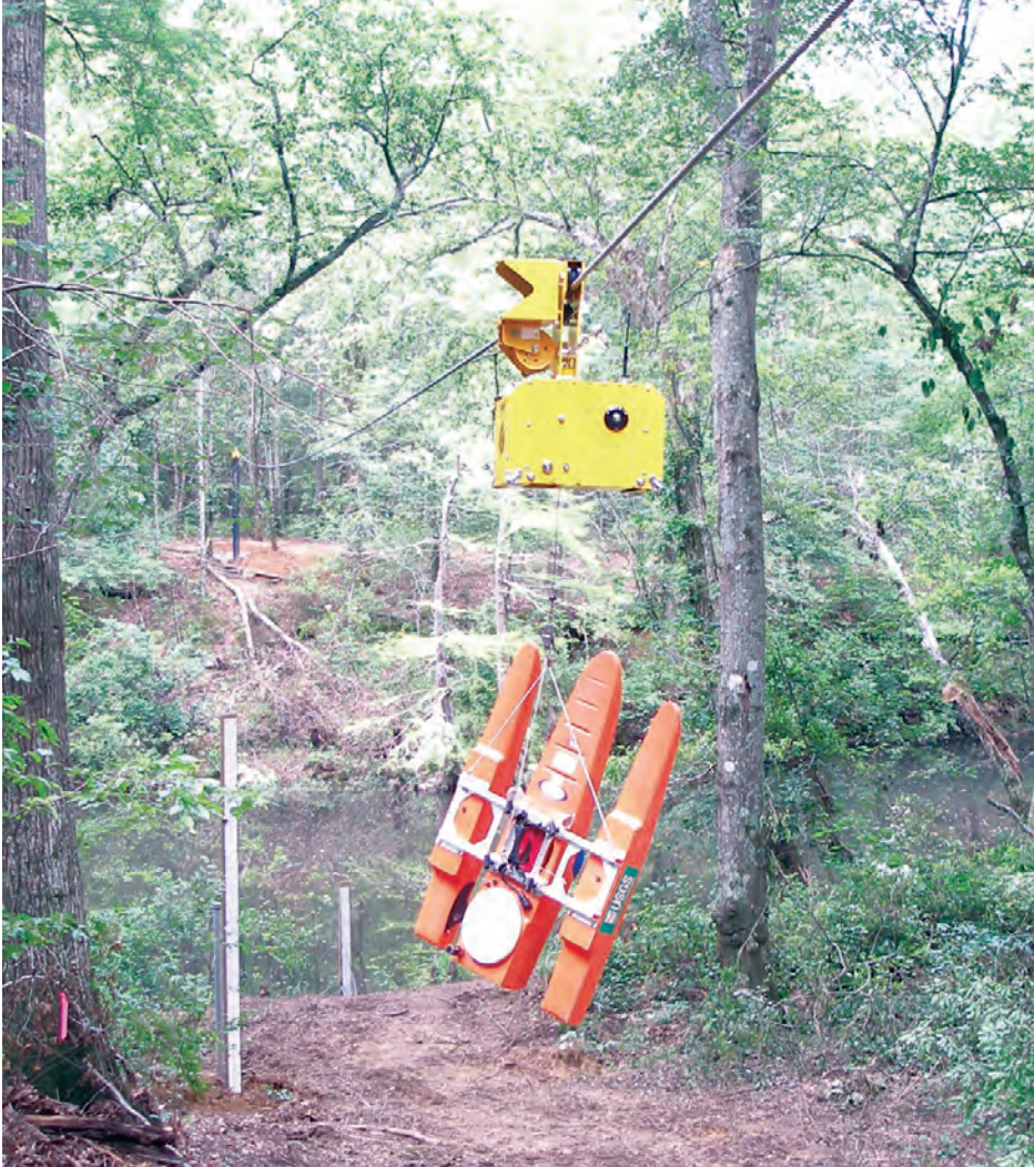
Figure 64. Remotely operated Hydrological Services Hornet cable carriage with ADCP and trimaran used by the USGS.
