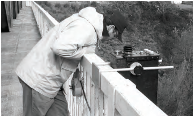
Figure 44. Hydrographer using an optical current meter to measure surface velocity.
