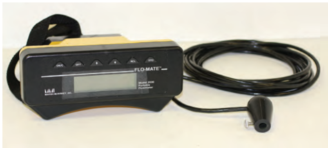
Figure 38. Marsh-McBirney Model 2000 electromagnetic flowmeter and display meter.
