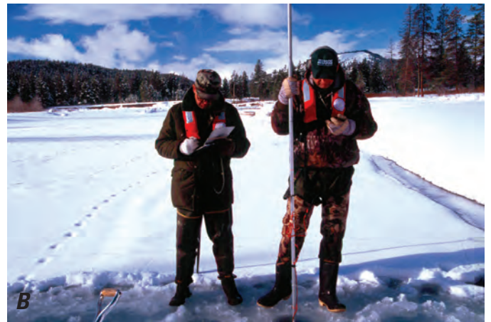
Figure 18. A, Ice drill being used to cut holes and B, ice rod being used to support current meter for a discharge measurement.
