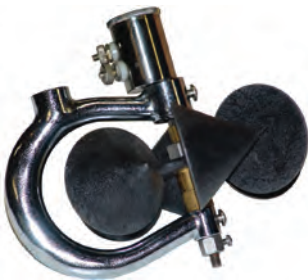
Figure 28. Price AA meter with winter-style yoke and polymer rotor.
