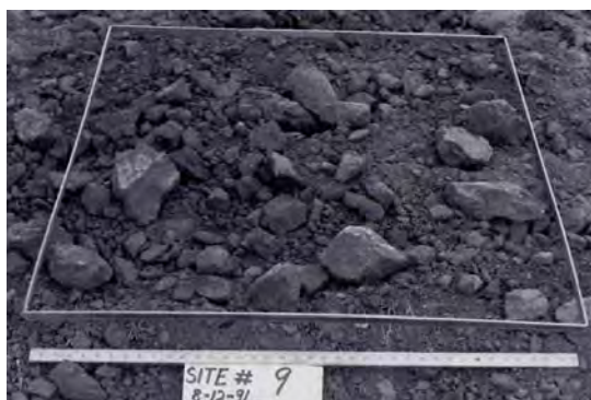
Figure 9.6. Soil surface with a 1.0 inch roughness just created by a mechanical disturbance.
