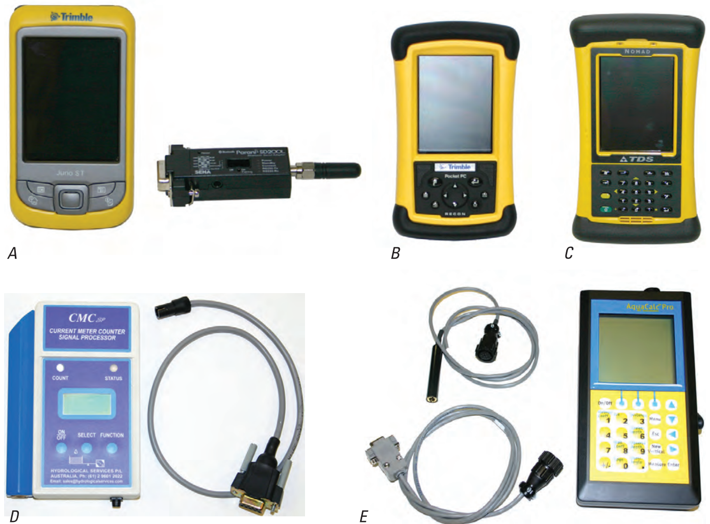
Figure 74. Personal digital assistants (PDAs) and electronic field notebooks (EFNs), clockwise from the top: A , the Trimble Juno SB PDA with GPS, Bluetooth, and Parani Serial Adapter; B , the Trimble Nomad 800 GL PDA with GPS and Bluetooth; C , the Trimble Recon PDA without GPS; D , the JBS Instruments Aquacalc Pro Discharge Measurement Computer; and E , the Hydrological Services Current Meter Counter Signal Processor with Bluetooth (CMCsp).
