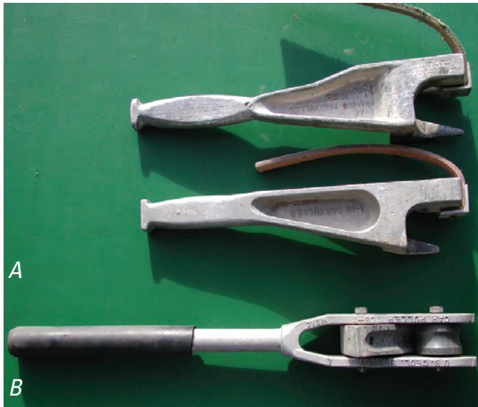
Figure 62. Cable-car pullers: A , with belt and B , with follower brake.
