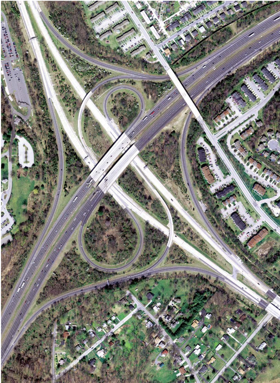
Figure 10-39. Directional Interchange with Semidirect Connection and Loops
