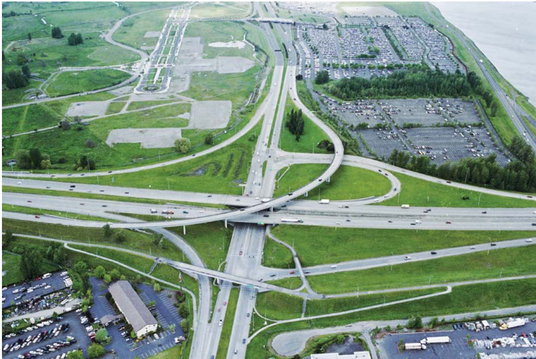
Figure 10-41. Four-Leg Interchange, Diamond with a Direct Connection
