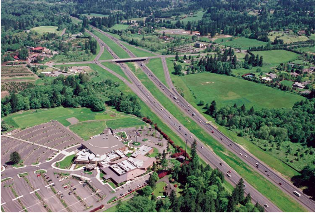
Figure 10-16. Typical Four-Leg Diamond Interchange
