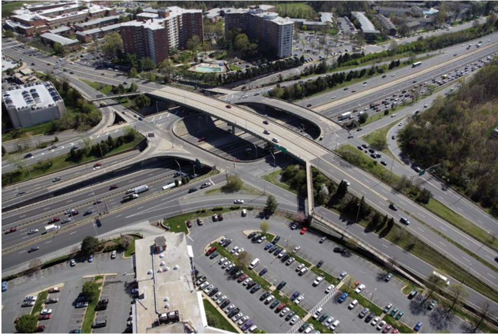
Figure 10-20. Freeway with a Three-Level Diamond Interchange
