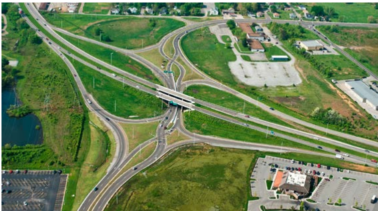
- B - Overpass DDI Source: Tennessee DOT
