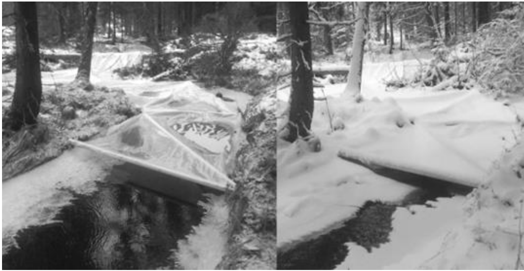
Fig. 2. Two photographs of the same downstream end of a section with artificial, plastic ice cover. During the course of winter, there were periods when light could penetrate through the artificial ice cover (left photograph) and periods when snow limited light penetration (right photograph).
