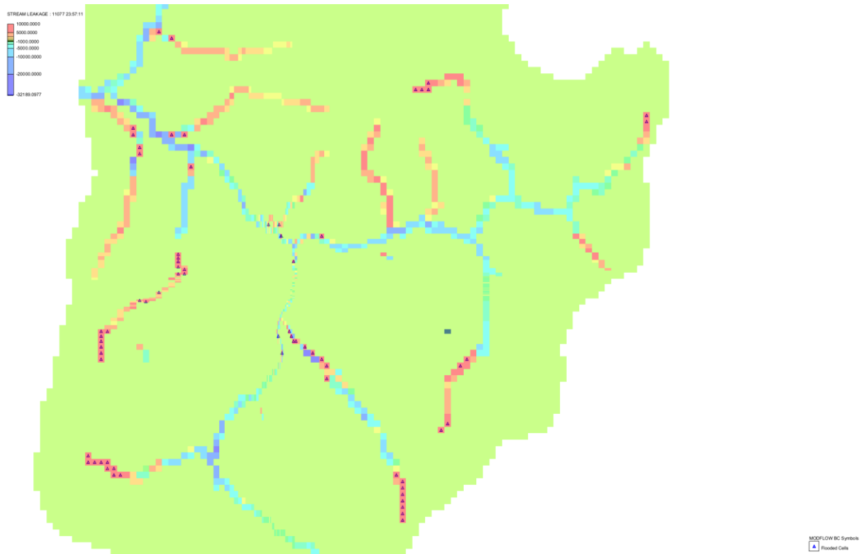
Figure 8. B&C 2018 EC Model SFR Stream Leakage (ft 3 /d) at 5/1/2012. Red areas show losing stream segments, while blue cells indicate streams are gaining.
