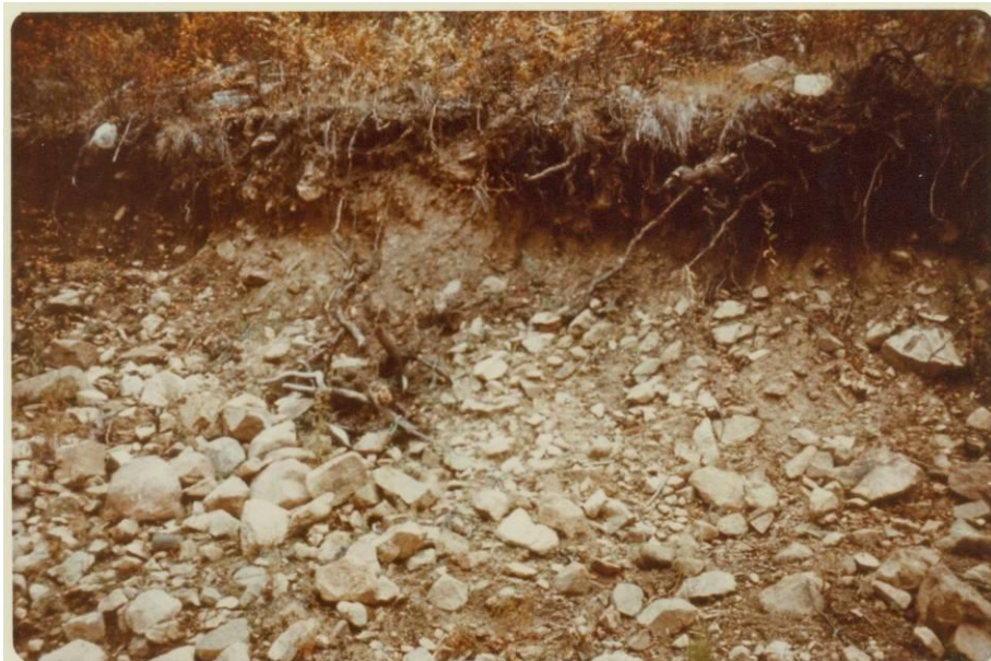
Competent rock fragments as shown in the above exposed profile aid the stability of cut slopes caused by road construction.
