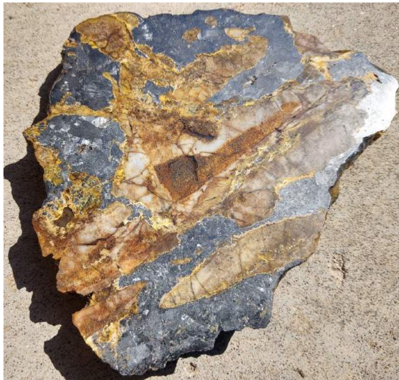
Figure 9-38: Sawn Hand Specimen Slab of Stibnite-Cemented Carbonate Breccia
