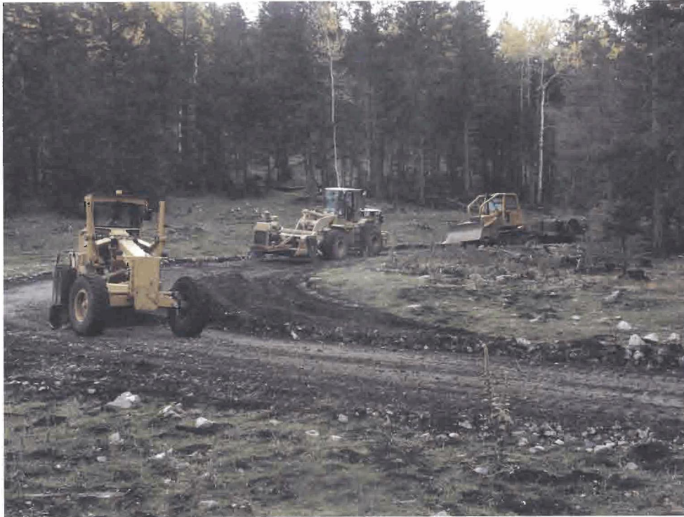
Figure 1. A grader (foreground), loader with rock crusher attachment (middle), and dozer with a grid roller attachment (background) were recorded during sound testing on the Lincoln National Forest, New Mexico on 22-23 October 2002 (see Appendix A).
