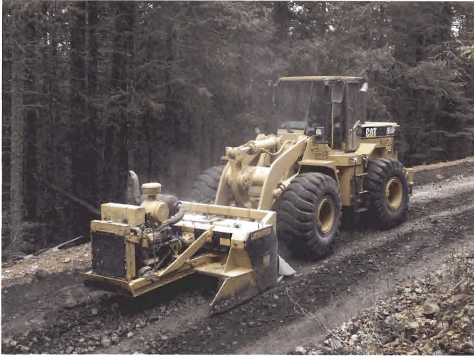
Figure A 1. Loader with rock crusher attachment used during sound testing on the Lincoln National Forest, NM, 22-23 October 2002.
