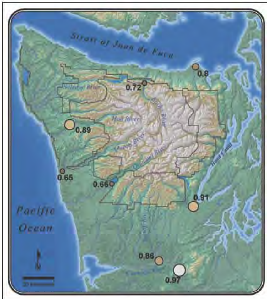
Figure 4.9—Projected decreases in low streamflows on the Olympic Peninsula. Numbers indicate the ratio of projected 20-year low streamflow statistics for the 2040s to 20 th -century low flow statistics under the A1B carbon dioxide emission scenario. Lower numbers, and smaller and darker red dots, indicate higher projected decreases in low flow. Olympic National Park and Olympic National Forest are outlined in dark gray. (Adapted from Mantua et al. 2010.)
