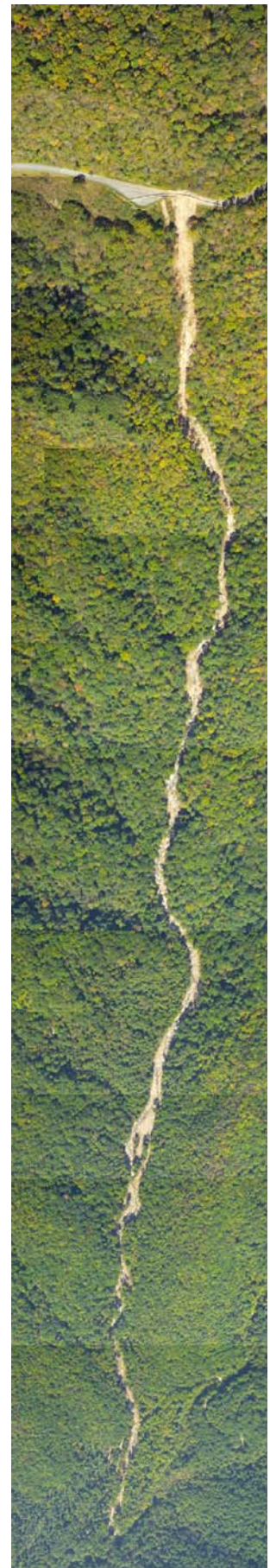
Fig. 3 Bear Drive Branch debris flow initiated at Blue Ridge Parkway fill-slope failure (Milepost 348) and traveled downslope 3 km (2 mi) across Pisgah National Forest, North Carolina (Hurricane Frances, September 8, 2004)
