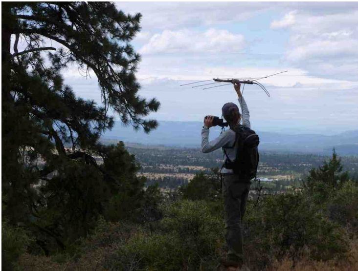
Figure 5. Using a receiver and antenna to assess the direction of a transmitter signal.
