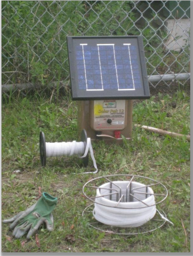
Some materials for setting up a portable electric fence.
