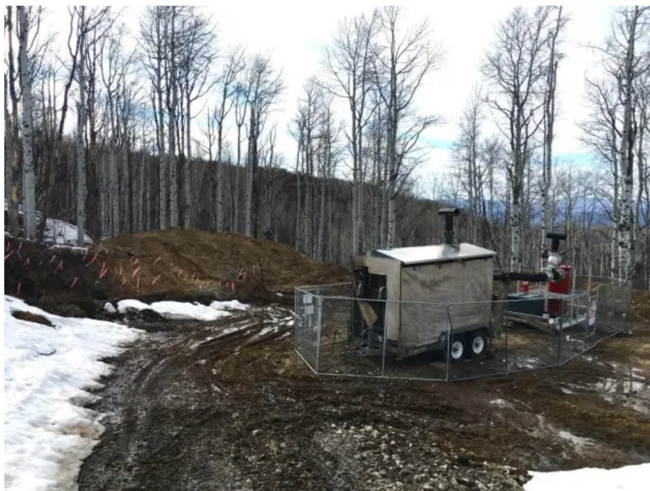
A methane exhauster above West Elk Mine. The gas it's venting can't be seen by the naked eye.
