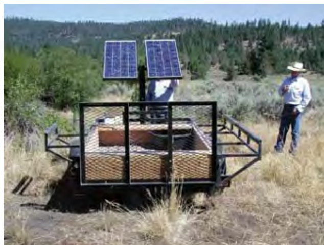
Figure 20. Mobile solar powered pump.
