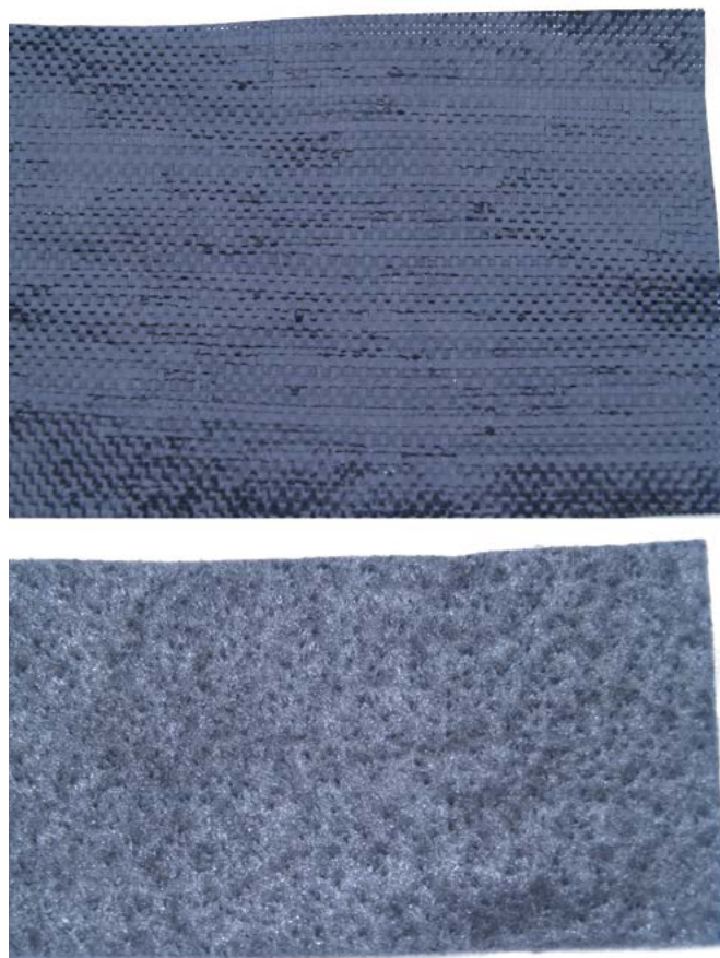
Figure 10.—Examples of woven (top) and nonwoven (bottom) geotextiles.
