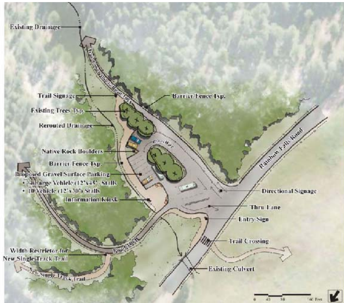
Figure 2-6: Illinois Gulch Parking Area Design
