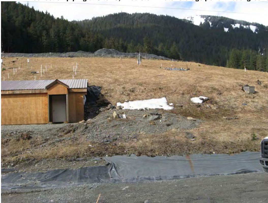
Photo 8: Frontal view of the test cover and wooden housing for seepage collection at Site 23; Active disposal of production rock in background
