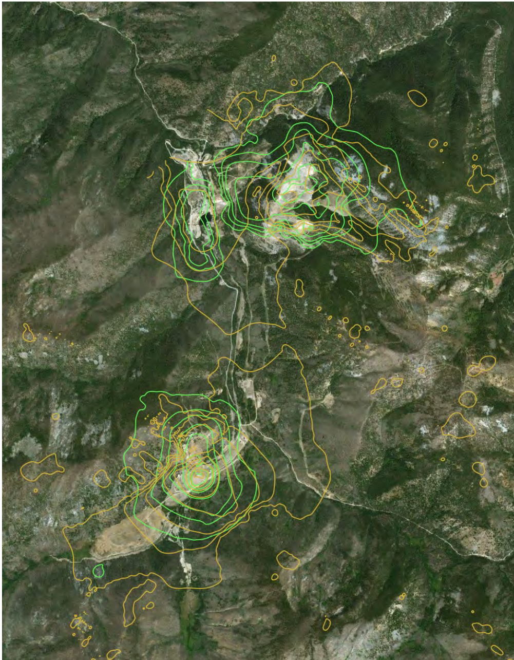
Figure 4. Simulated drawdown at mine year +12 (model time = 14 years), for the provided Proposed Action model (green), and CA Test 1 (yellow) for drawdown 5 feet and greater.
