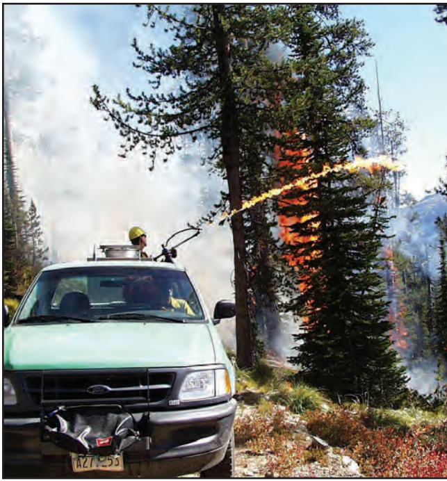
Figure 4.18. Prescribed fire ignition is being implemented in a whitebark pine restoration site using the terra-torch.
