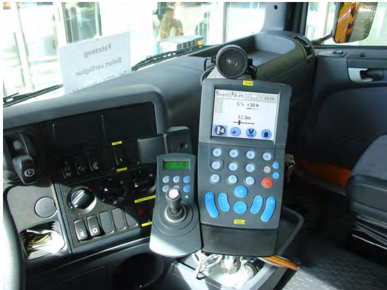
FIGURE 10 Control panel to control gritters and snowplows with integrated data recording and route guidance.
