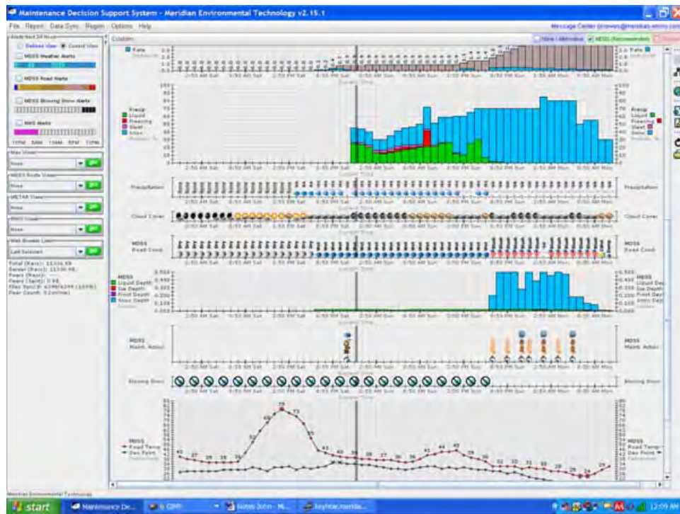
FIGURE 5 MDSS route view showing past conditions and forecasted conditions.
