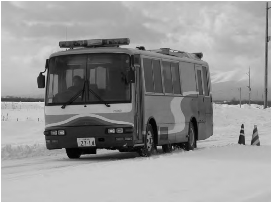
FIGURE 2 Bus-typed locked-wheel friction tester.
