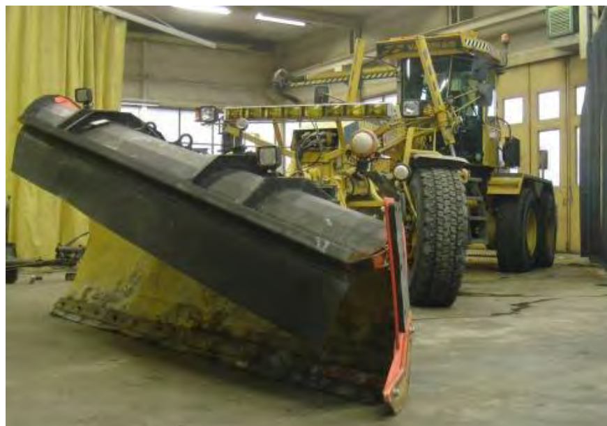
FIGURE 9 Grader with front-mounted plow and plowshare.
