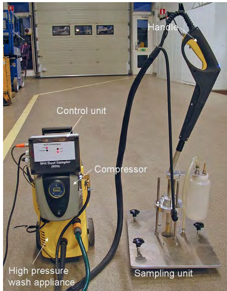
FIGURE 1 Overview of the WDS electrical appliances ( left ): the high-pressure wash appliance, the compressor, and the control unit. The sampling unit is shown at the right.
