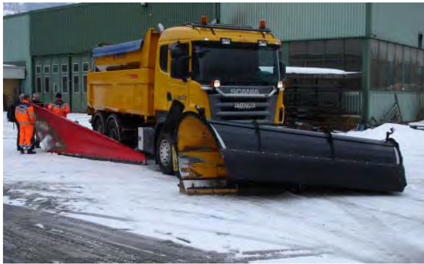
FIGURE 8 Truck with spreader in front-mounted plow and side-mounted plow.
