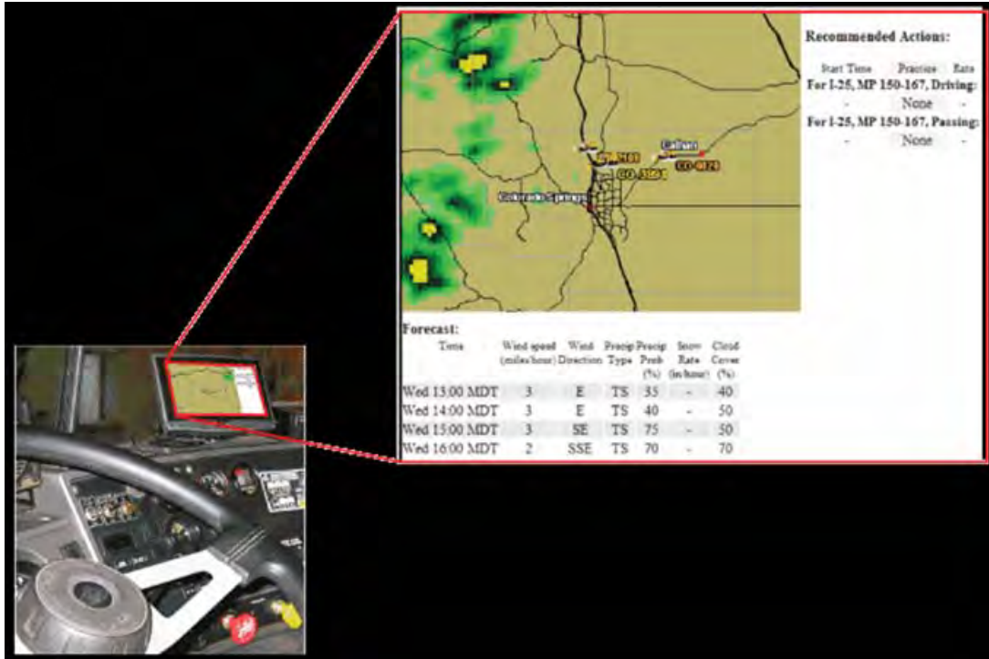
FIGURE 6 In-vehicle truck display of MDSS recommendations.
