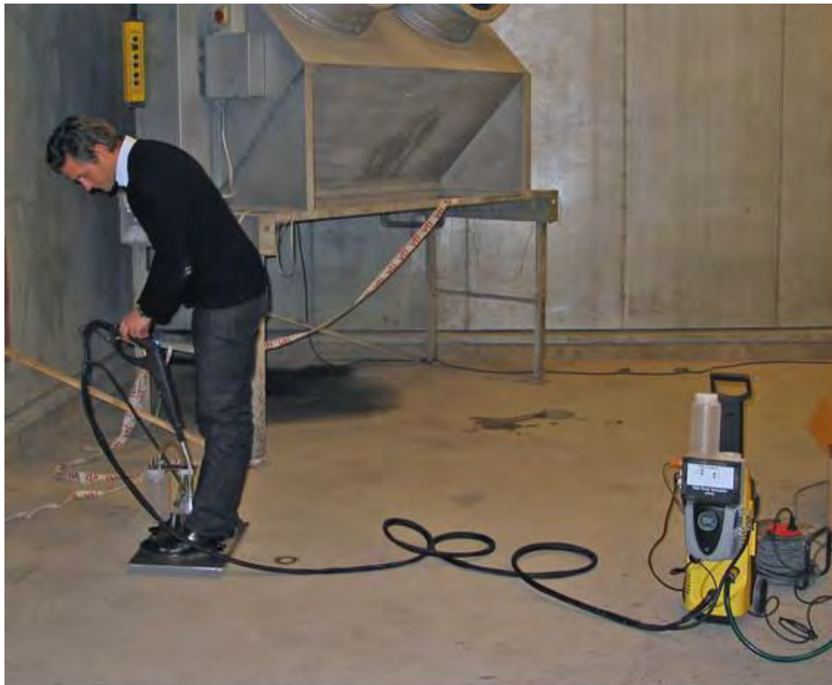
FIGURE 4 The WDS during sample retrieval.
