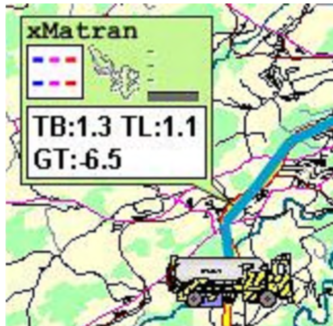
FIGURE 7 Example of the display of a measuring point flag and deployment vehicle with current data on the dynamic map.
