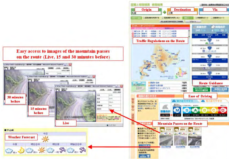
FIGURE 16 Easy access to images of the mountain passes on the route (new distance and travel time search function of Northern Road Navi website).
