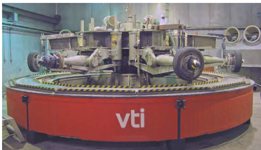
FIGURE 1 The Swedish National Road and Transport Research Institute circular road simulator.
