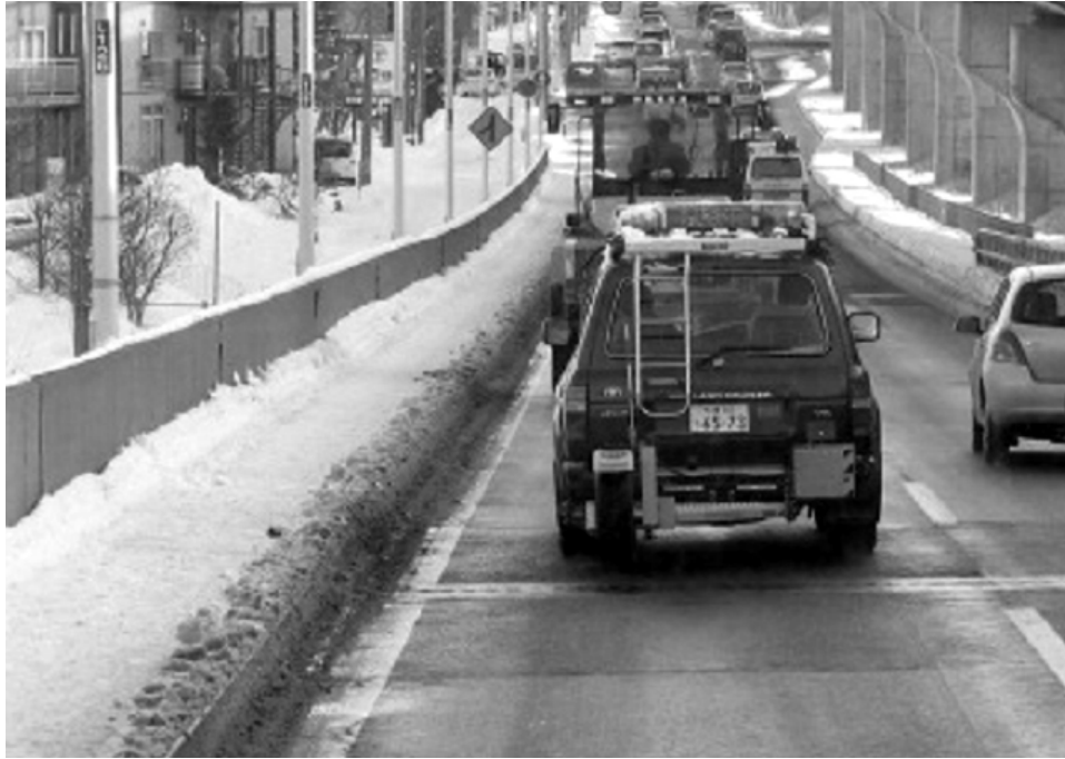
FIGURE 10 Examination of road condition by continuous friction tester.
