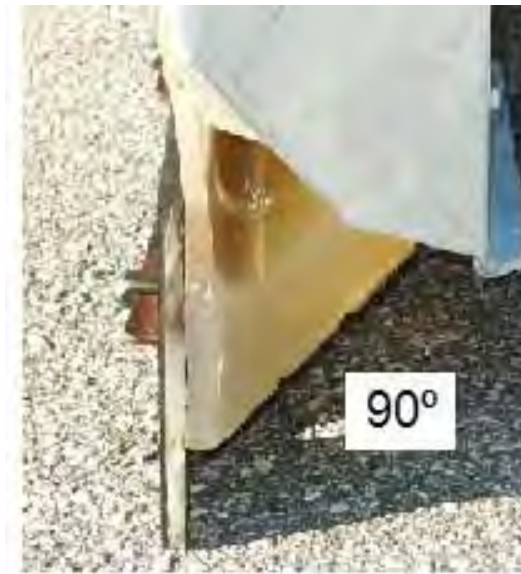
FIGURE 5 New cutting edge, 90-degree angle.
