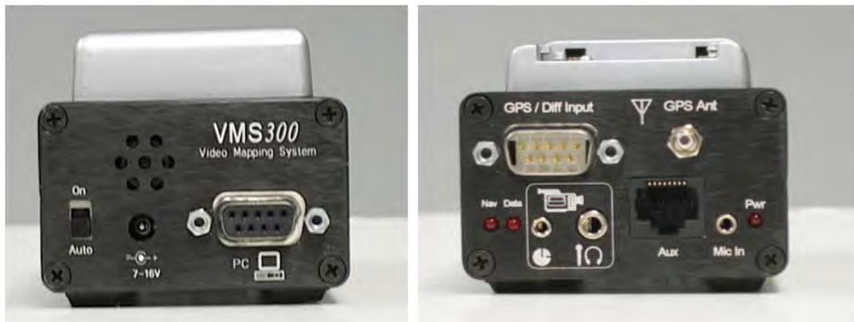
FIGURE 4 Front and rear views of RedHen GPS–video unit. Input and output ports for a laptop, GPS antenna, telephone, microphone, and video camera are shown.
