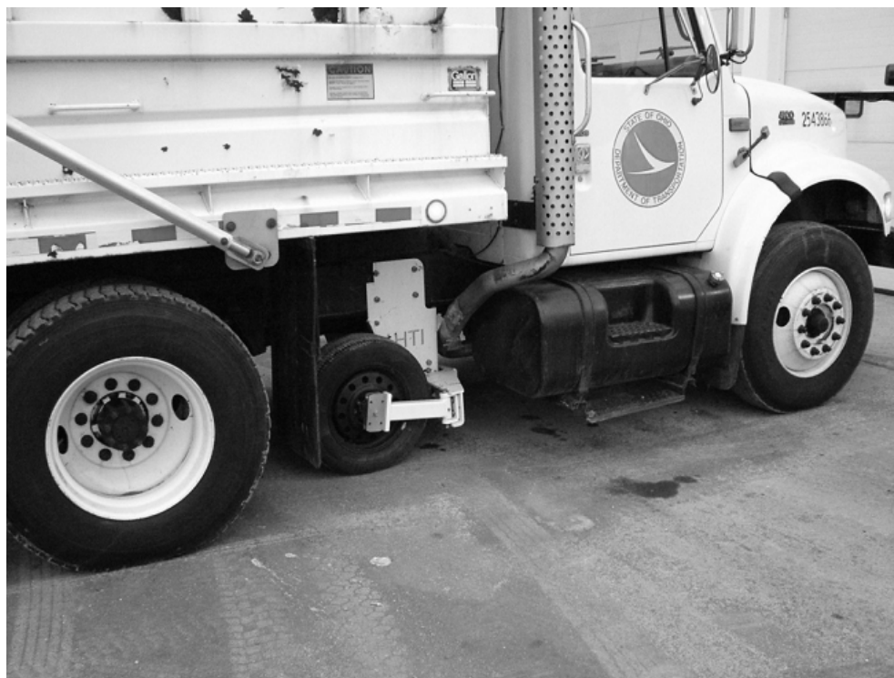
FIGURE 4 Anti-icing operation vehicle with continuous friction tester (Ohio DOT).
