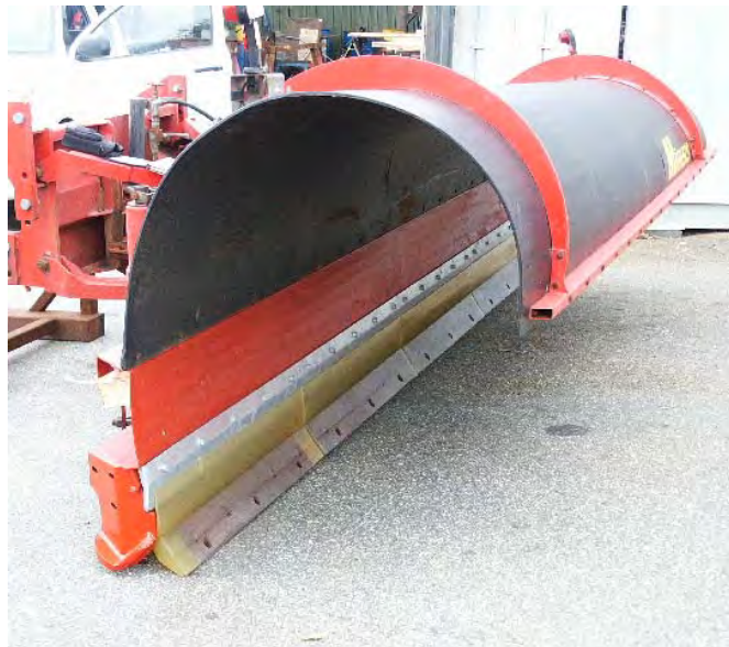
FIGURE 3 Snowplow with modified cutting edges.
