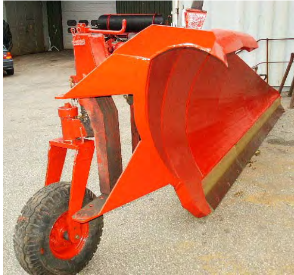
FIGURE 4 The wheel on the side plow will be replaced with a wheel made out of polyurethane.
