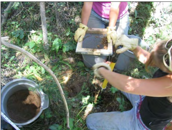
Figure 6.25. Collecting and sieving soil samples in the field.
