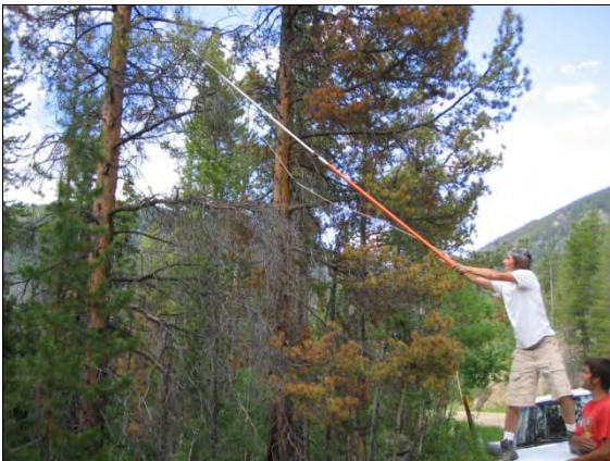
Figure 6.28. Collecting foliar samples with a pole pruner.
