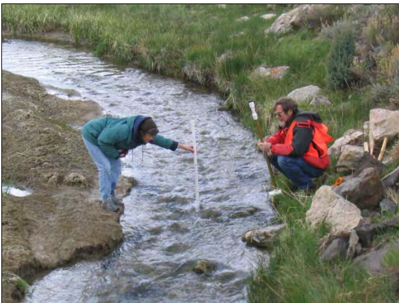
Figure 6.30. Measuring stream depth and water flow in the field.
