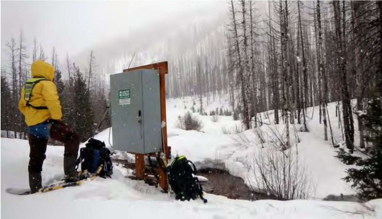
USGS Hydrologic Technician Alvin Sablan prepares to check the USGS stream gage on Meadow Creek in the historical Stibnite Mining District of central Idaho. USGS photo
