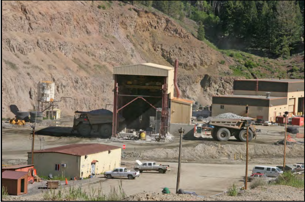
Photo 2.1-4. Primary crusher being fed by haul trucks loaded with ore.
