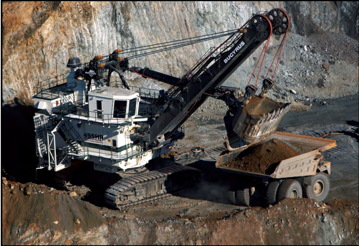
Photo 2.1-2. Electric shovel, 40 cubic yard bucket.
