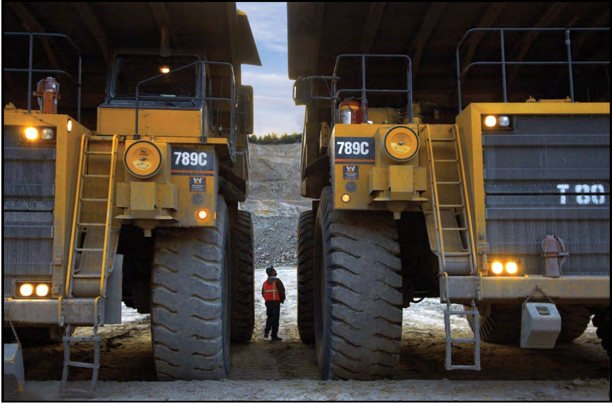
Photo 2.1-3. Haul trucks, 200 tons.
