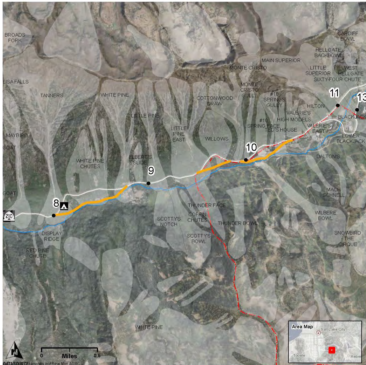
Figure 3-3. S.R. 210 Realignment for Avalanche Mitigation
