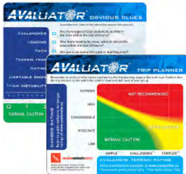
Figure 7. The Avaluator decision support pocket card. On one side, the trip planner uses the ATEs rating and the avalanche danger to inform users of travel recommendations. On the other side a checklist of obvious clues prompts the user to look for danger signs and aids in slope evaluation by making travel recommendations.
