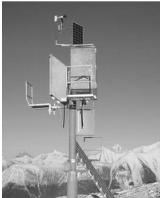
Figure 4. An Avalanche Guard protecting the Trans-Canada Highway near Revelstoke, British Columbia. Photographer: British Columbia Ministry of Transportation Snow Avalanche Program.
