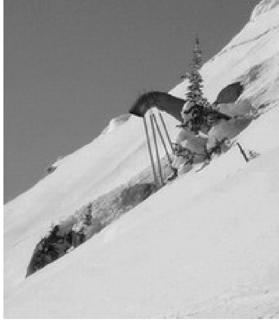
Figure 3. A GazEx exploder near Kootenay Pass, British Columbia. Photographer: British Columbia Ministry of Transportation Snow Avalanche Program.
