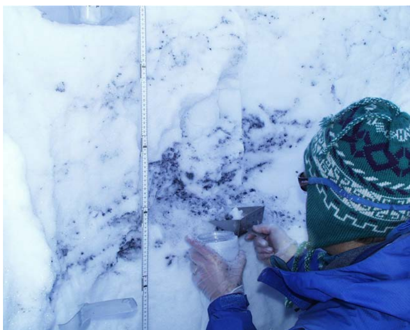
Figure 7. Black areas in snow characteristic of blast zones created by explosives used for snow avalanche control, The Canyons ski area, Utah, February 15, 2001.
