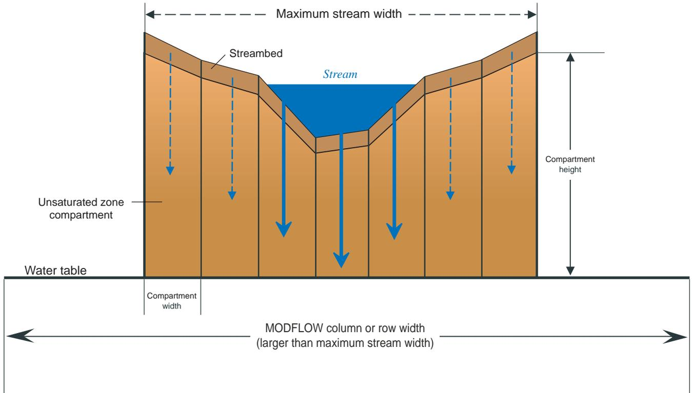
**Figure 3.** Discretization of unsaturated zone beneath a stream in a single MODFLOW cell. The unsaturated zone is discretized into seven compartments defined by eight points in this example. Dashed lines represent stream depth and infiltration when stream is at maximum width.
