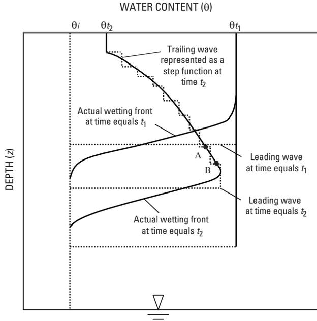
**Figure 2.** A wetting front through a uniform column of unsaturated material affected by a decrease in surface flux and results from a kinematic-wave approximation of the wetting front using leading and trailing waves. (Modified from Smith and Hebbert, 1983.)
