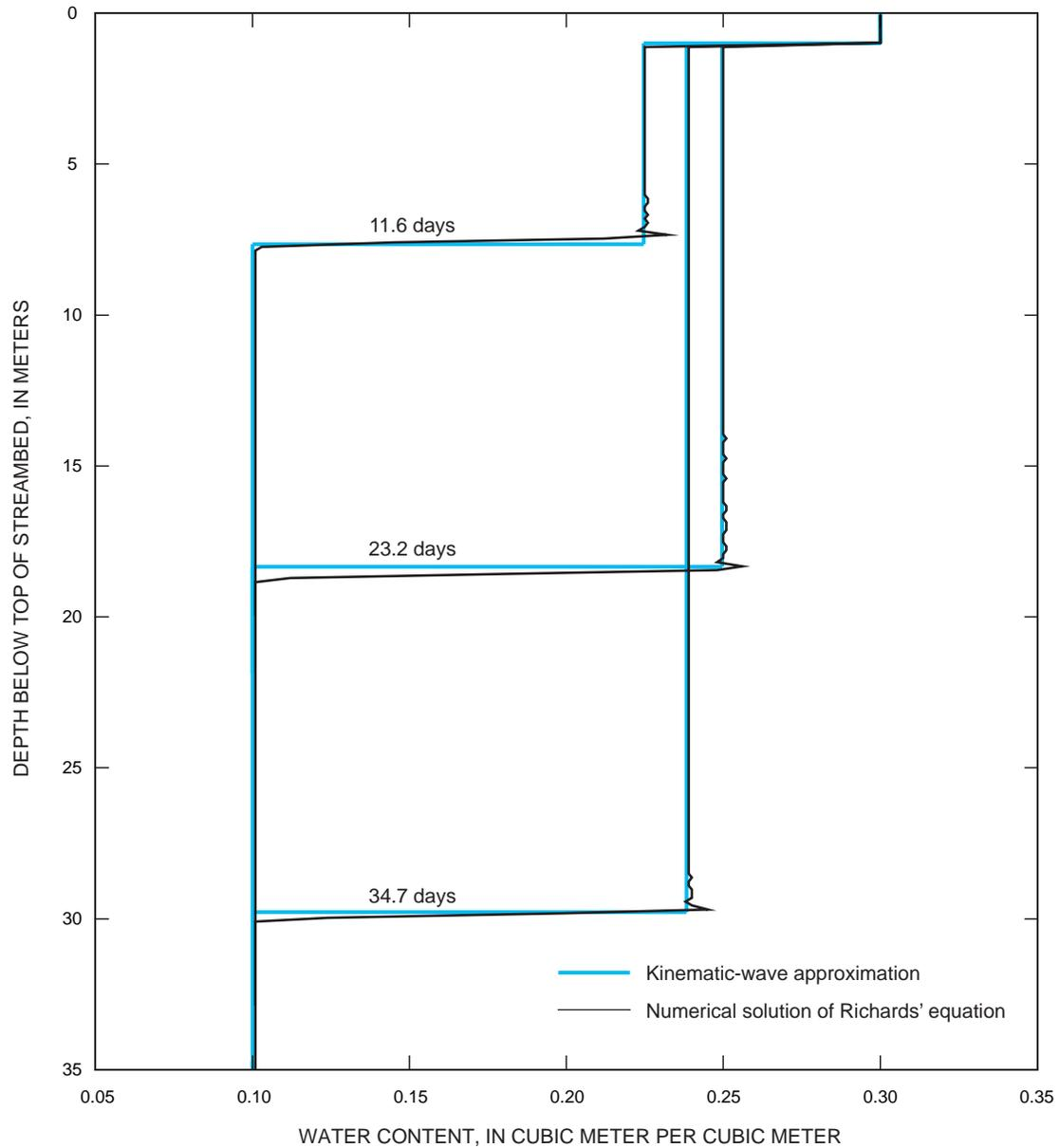
**Figure 5.** Comparison of results from the kinematic-wave approximation in the Streamflow-Routing (SFR2) Package with the Variably Saturated Two-Dimensional Flow and Transport (VS2DT; Healy, 1990) Model for seepage through a one-dimensional column filled with a silt loam. Variations in water content below the streambed (thickness of 1 meter) are the result of different calculated flux rates across the streambed caused by varying stream depth (from Niswonger and Prudic, 2004, fig. 4).
