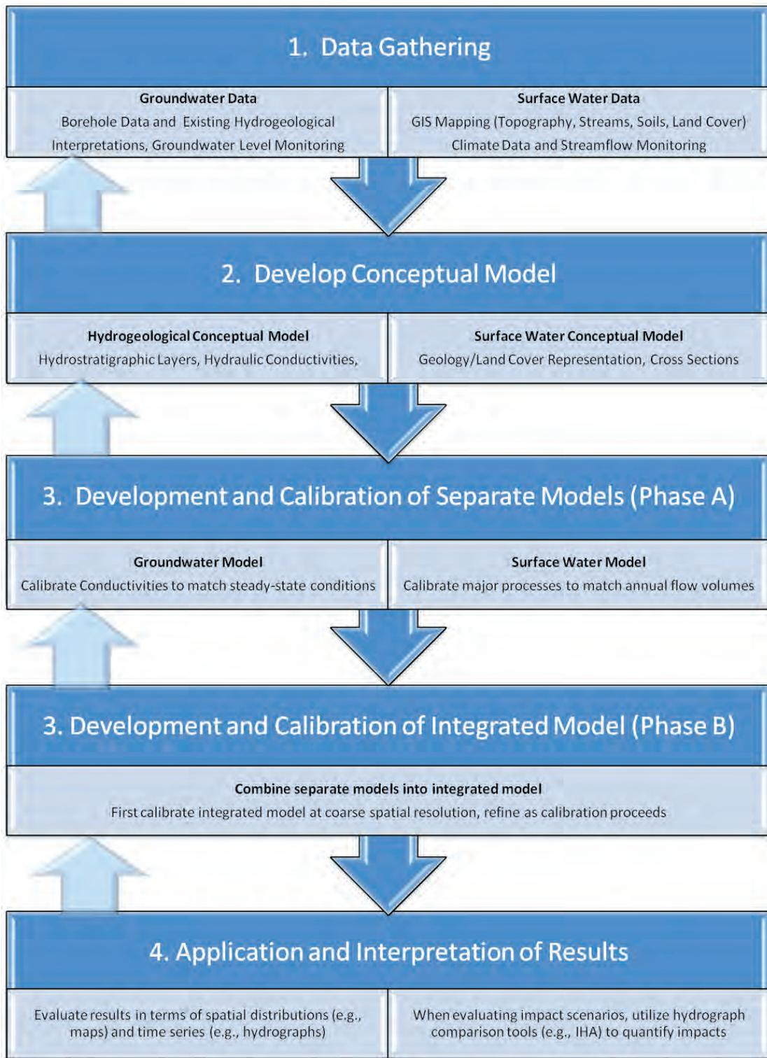
Figure 5.1 Phased Approach for Integrated Model Applications
