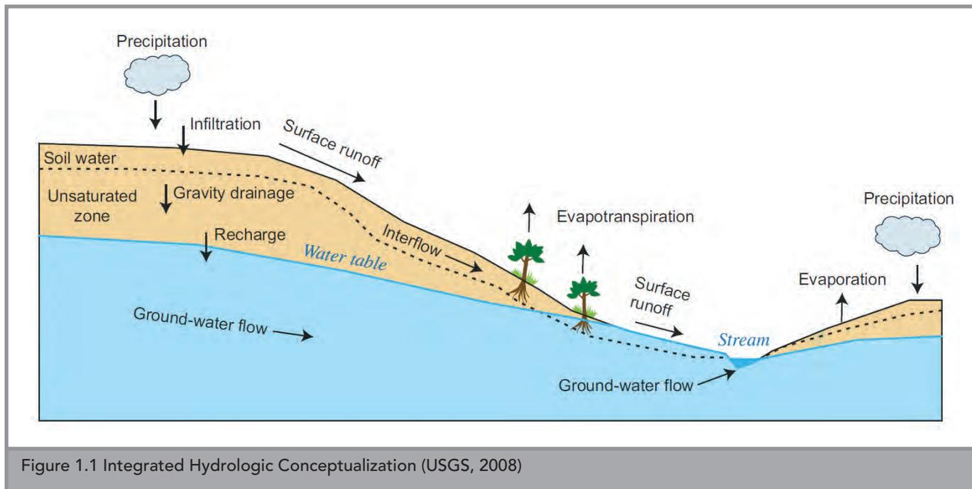
Figure 1.1 Integrated Hydrologic Conceptualization (USGS, 2008)
