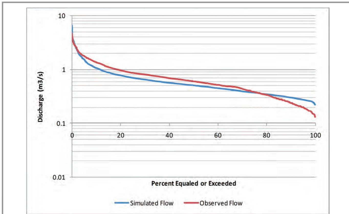
Figure 4.9 -Mill Creek at Side Road 10 - Flow Duration Curve (April - Dec)
