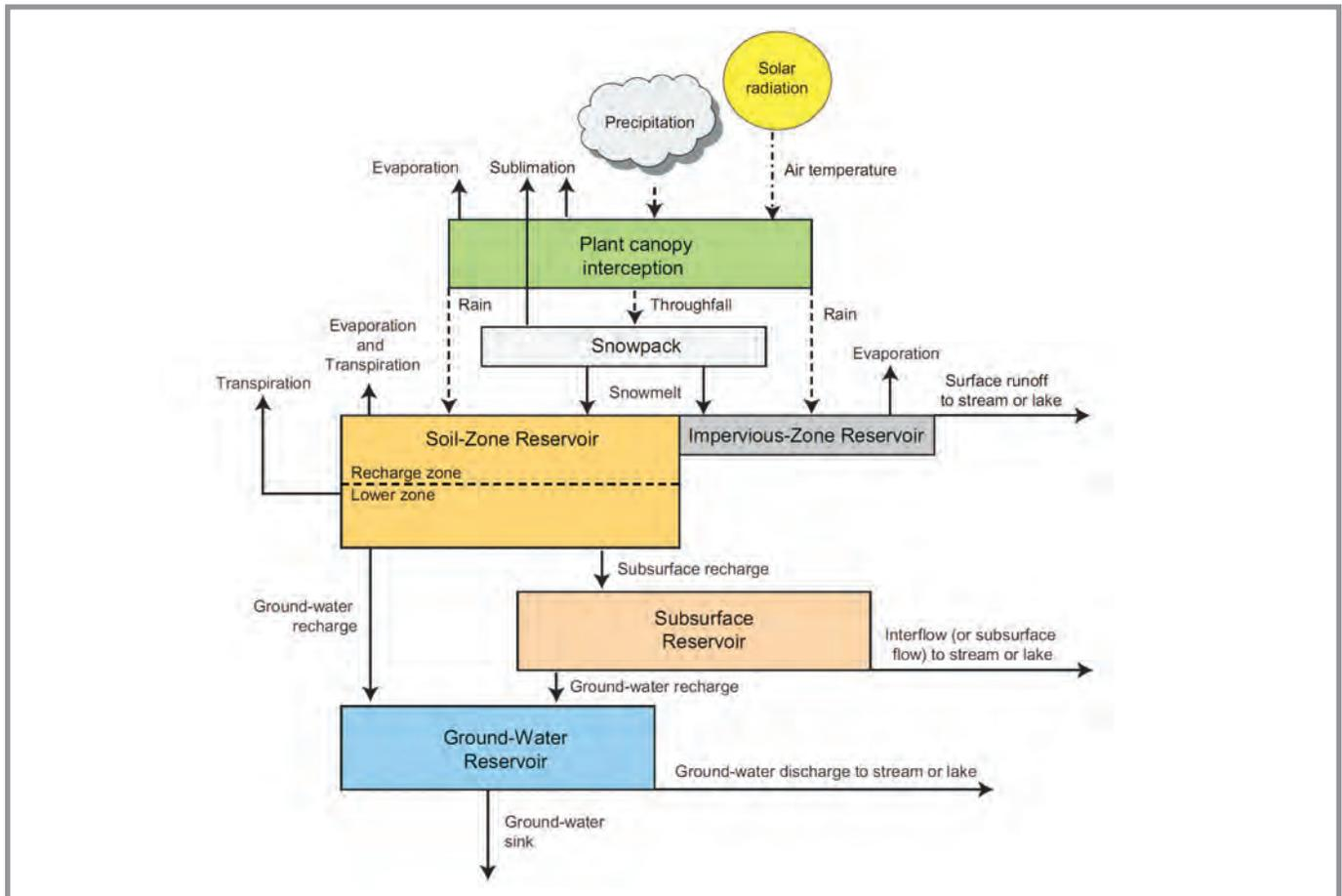
Figure 2.2 PRMS Process Schematic (Source: USGS, 2008)
