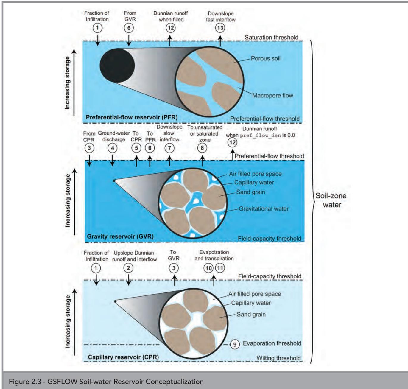
Figure 2.3 - GSFLOW Soil-water Reservoir Conceptualization
