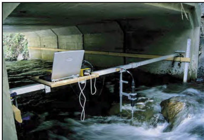
Figure 3A. ADV harness in culvert 2 inlet region.
