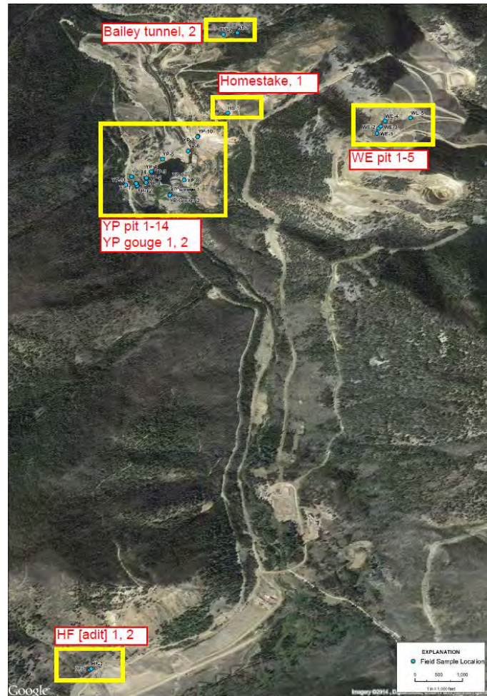
Figure 5. Surface samples. Yellow squares highlight where groups of samples were collected, numbers refer to the number of samples collected at each site. Source: SRK 2017 Baseline Geochem Fig. 3-4
