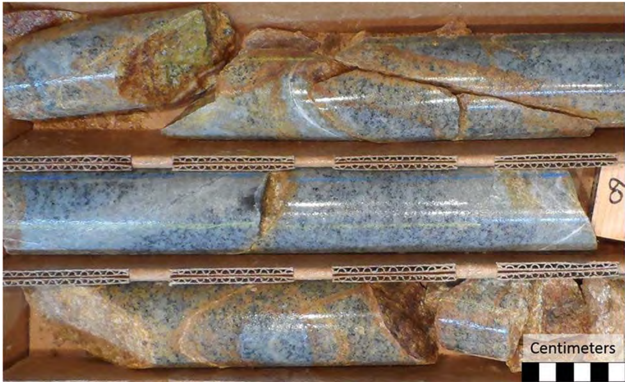
Photograph 7.4: Example of the Biotite Granite in HQ Core with Local Fe Oxide
