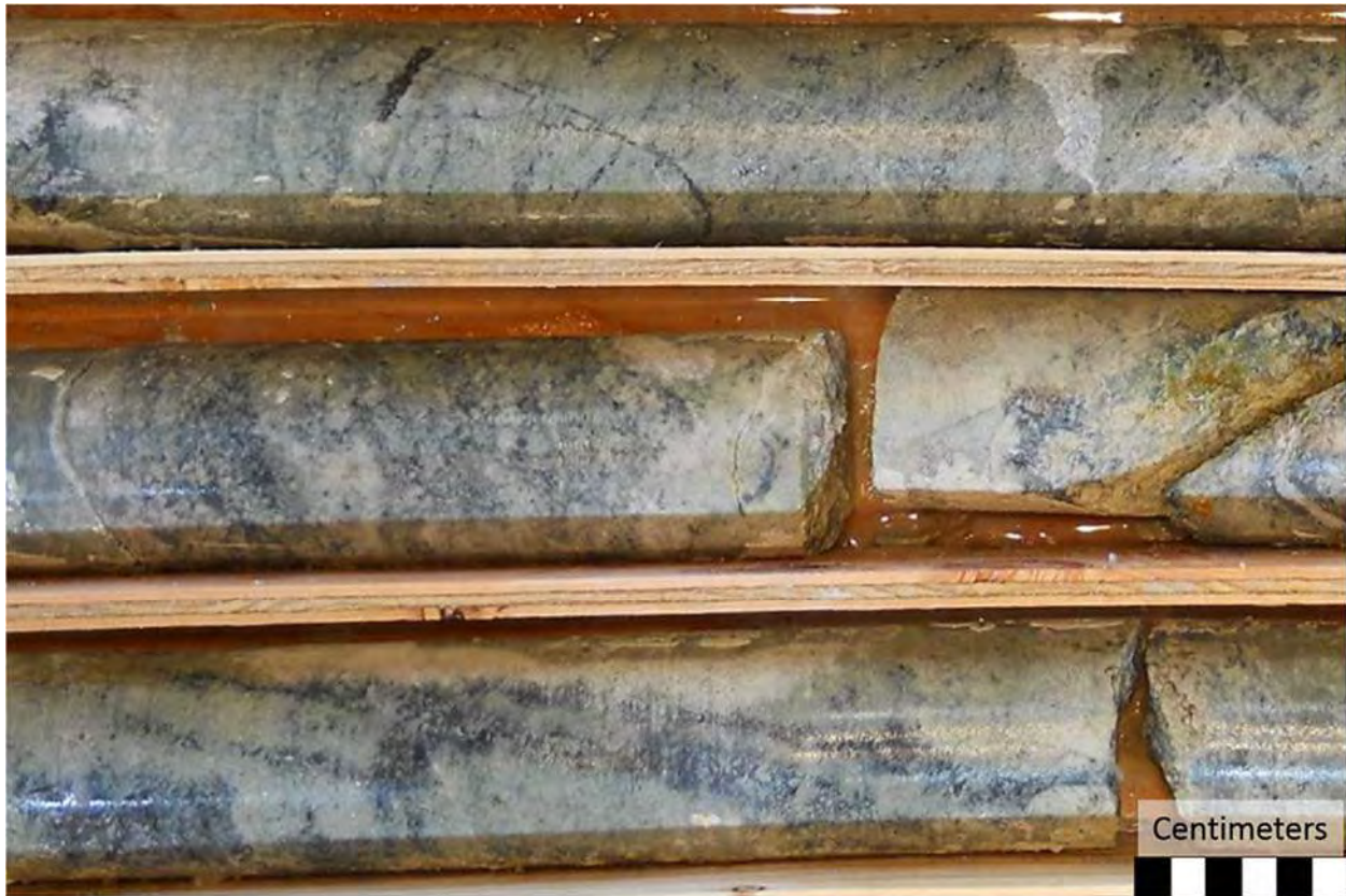
Photograph 7.11: Example of the Lower Calc-Silicate in HQ Core
