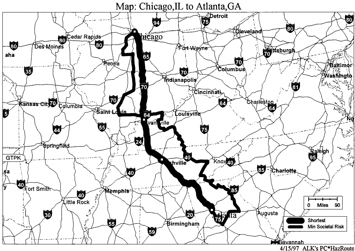
Figure 10a. Shortest path and minimum societal risk path for the Chicago-Atlanta pair.
