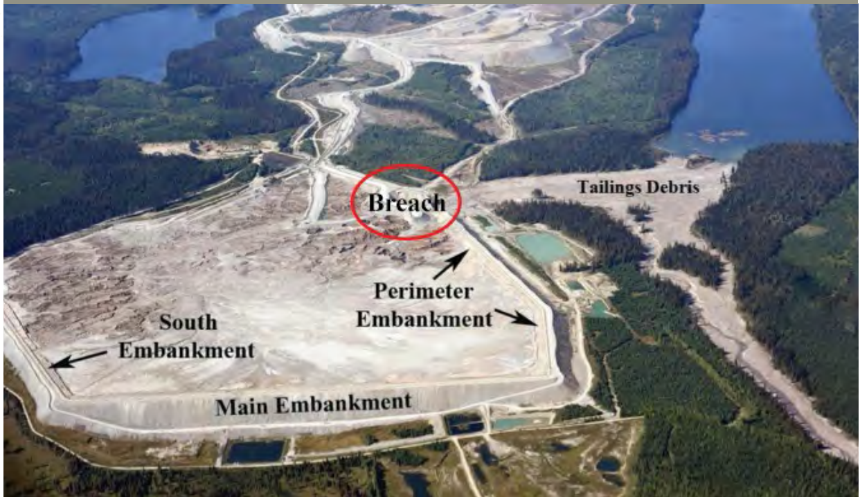
Exhibit 17: Description of Mount Polley dam embankments
