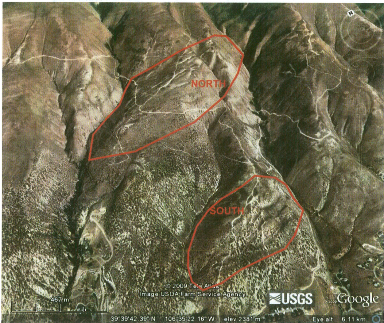
Fig. 2. Google Earth oblique view to the north of the two landslide polygons mapped by Colton et al. (1975). Each polygon contains a swarm of anomalous NE-SW ridges and troughs, some of which cross-cut other landforms such as gullies and swales.
