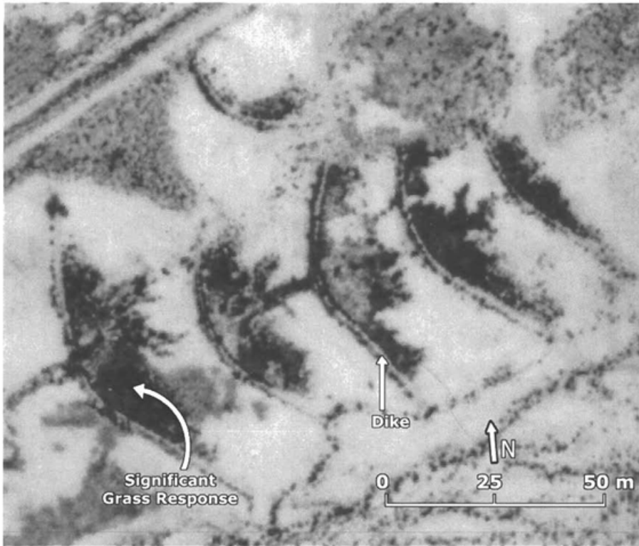
Fig. 14-2. Aerial photo (1998) of contour dikes constructed in the 1970s showing vegetation establishment.
