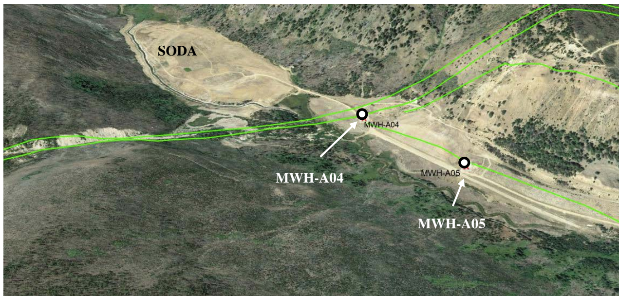
Figure 4. Location of alluvial wells with elevated dissolved Hg at old heap leaches Looking up Meadow Creek Valley; MWH-A01 is located above SODA (outside of image). Green lines represent fault lines. Both wells are in the location of the future HF pit. Geo-location of well and fault lines relative to land features contributed by B. Prucha.
