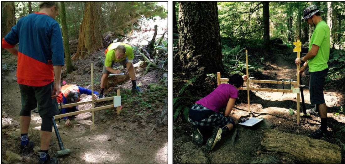
Figure 3. CSA measurements along the test trail loops at permanent sampling stations.
