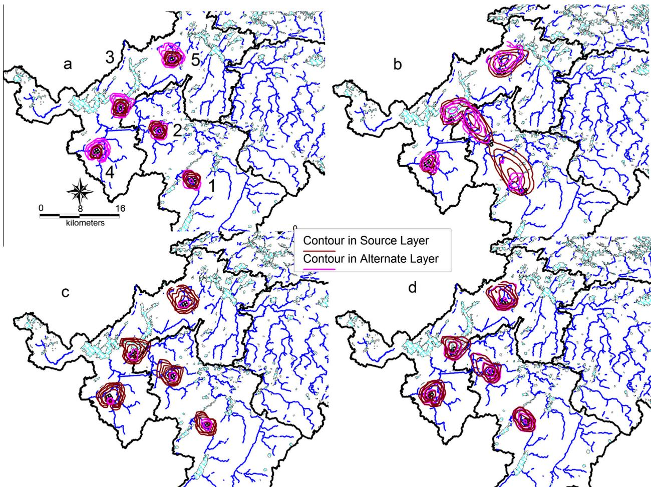
**Fig. 10.** Concentration contours for (a) underground source after 10 years, (b) underground source after 1000 years, (c) surface source after 10 years, and (d) surface source after 100 years. Underground source is layer 3, surface source is layer 1. Alternate layer is layer 1 in (a) and (b), layer 3 in (c), and layer 2 in (d). The contaminant source number is shown in (a). Contours range from 1 to 100,000  $\mu\text{g}/\text{l}$  from outer to inner.
