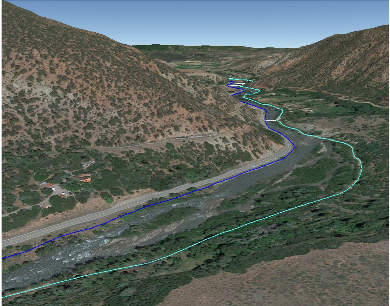
Figure 5 The Red Wind Point section is another example of the transitional confined valley and river type. Alignment B follows the abandoned railroad grade which runs up the right riparian area, effectively isolating a portion of the floodplain and riparian area from the river. If the railroad line is not repurposed, it could potentially be remediated for river and riparian restoration.
