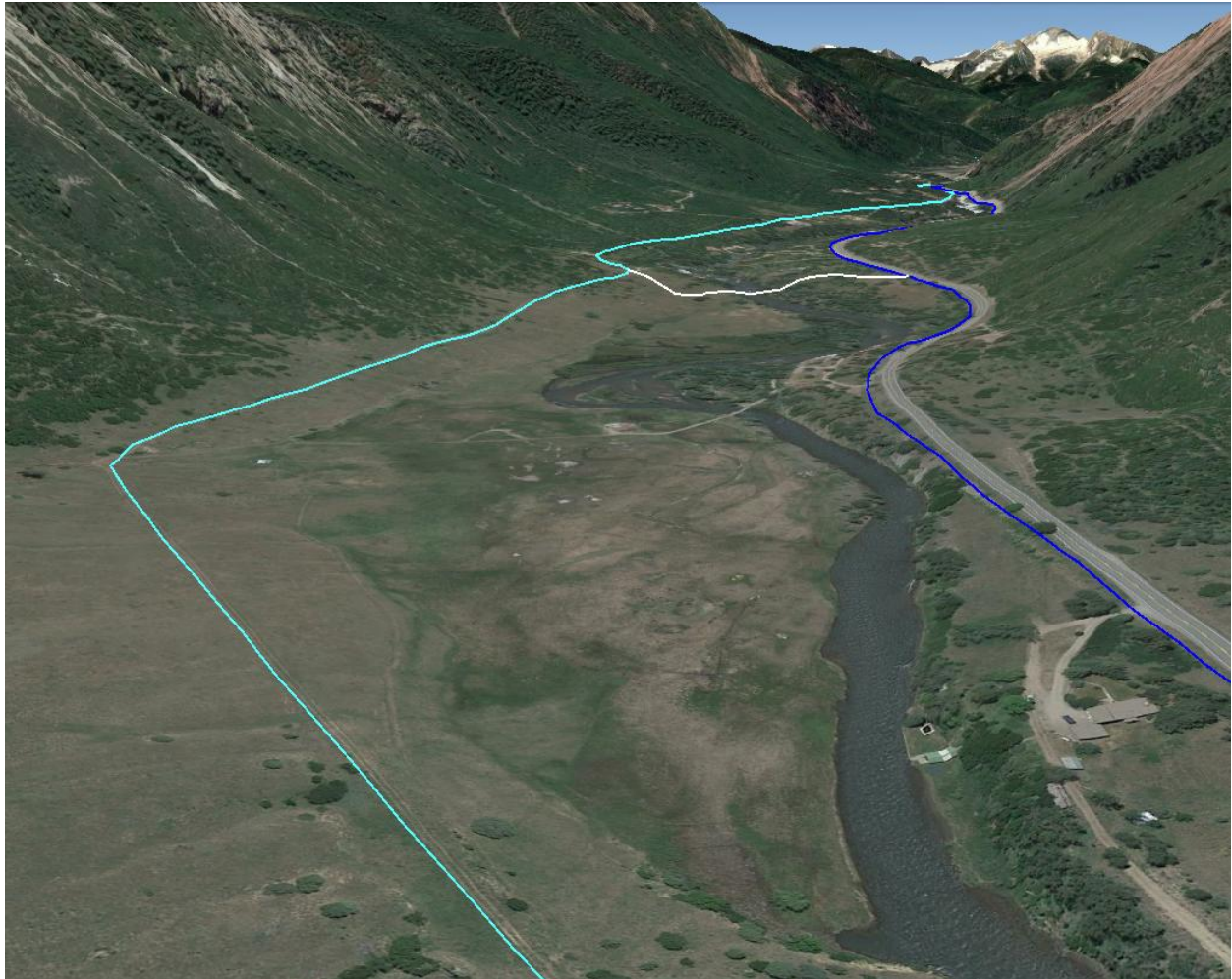
Figure 11 Looking upstream at the Filoha section where the river in the foreground is channelized and riparian vegetation on the east side (left in photo) has been cleared for agricultural use. Alignment B follows the old rail line on the upland hillslope above valley bottom.
