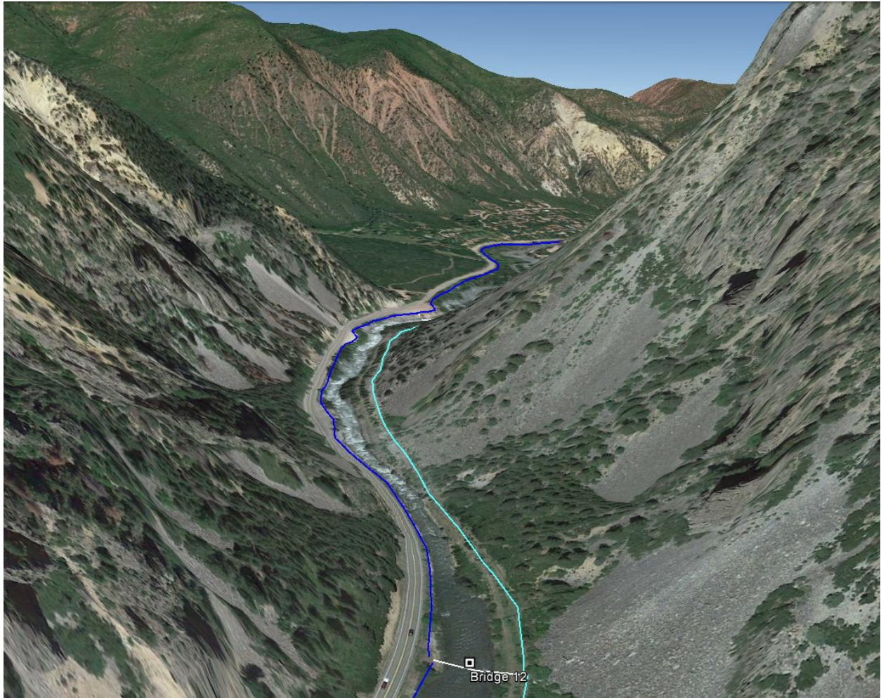
Figure 1 A typical reach through a very confined valley on the Narrows section. Encroachment and armored banks from Highway 133 (left) and the abandoned railroad (right) extend the length of this reach. Bridge option 2 is in the foreground.
