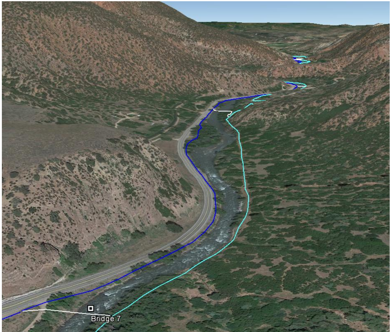
Figure 2 Typical confined reach on the Andrews section. The photo shows encroachment on the left where Highway 133 is constructed on armored fill on the valley bottom in the riparian zone and the abandoned railroad line on the right. Trail Alignment A follows the highway and B follows the railroad line. Bridge option 7 is in the foreground, and bridge option 6 is farther downstream.
