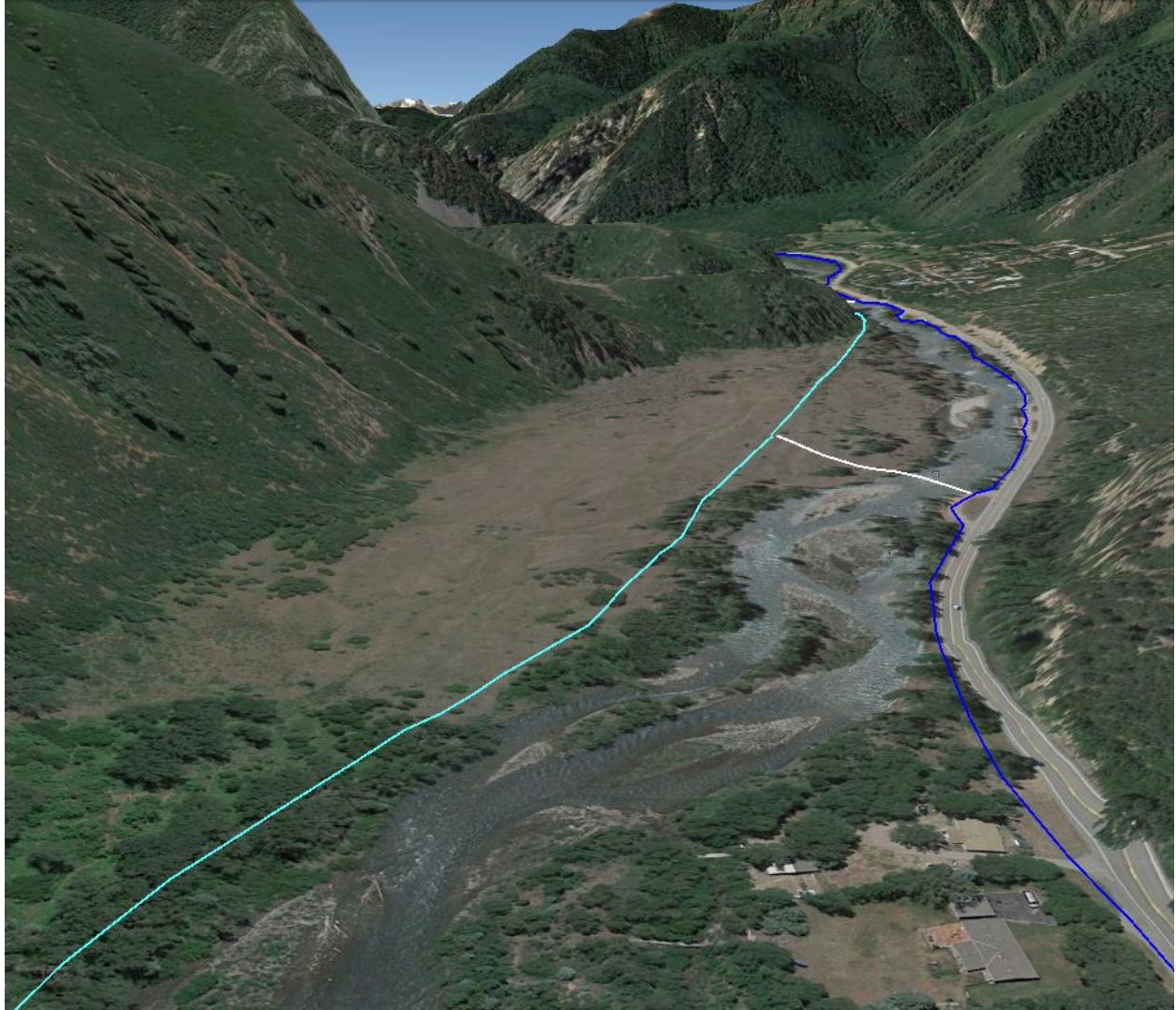
Figure 12 On the Janeway South section, riparian vegetation was cleared from the east side riparian area (left in photo) which is also disconnected from the river by the abandoned railroad line that runs through the center of the valley bottom. Routing the trail along this line in Alignment B would probably eliminate river and riparian restoration potential on this impaired reach.
