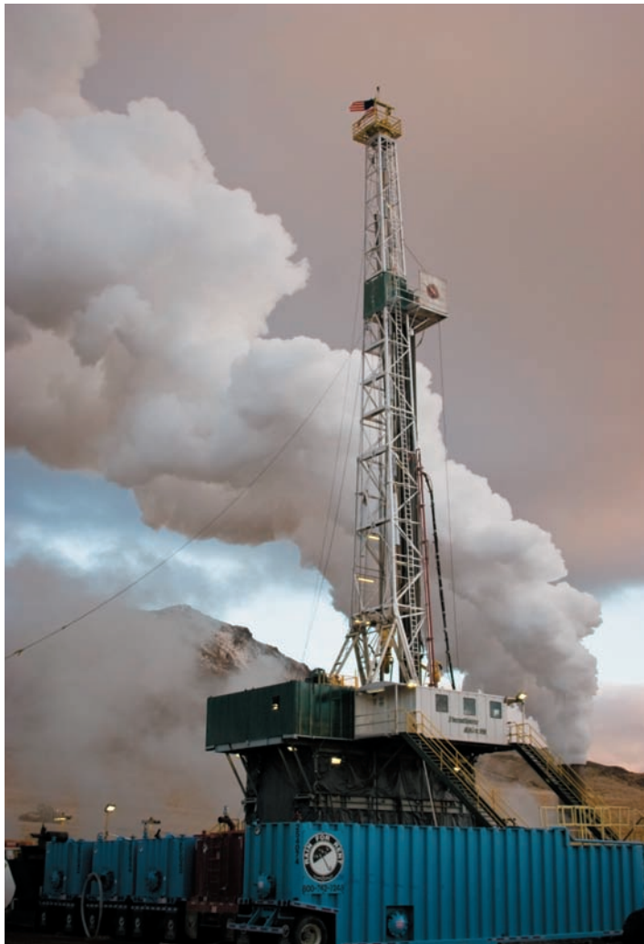
A flow test in progress at the Blue Mountain Geothermal site. The initial drilling of the wells may occupy only 2-3 acres, but this is the phase where most disturbance occurs. Photo courtesy of Bureau of Land Management, Nevada State Office.
