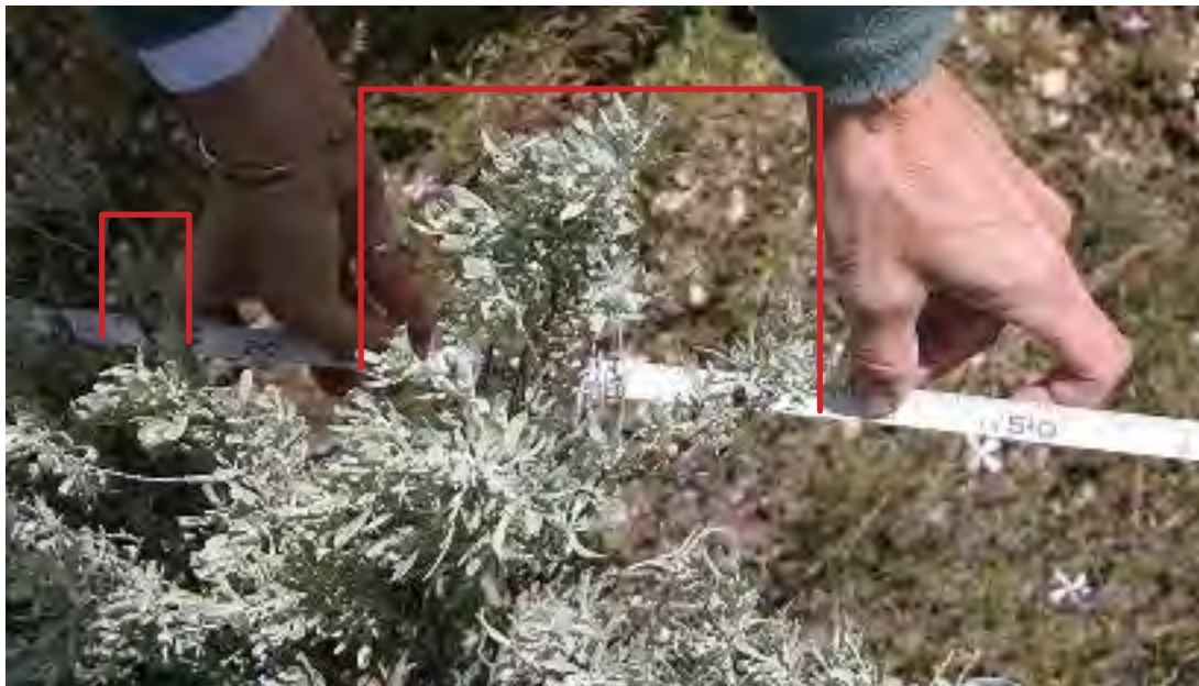
Figure B-5. Measuring shrub canopy cover using the line intercept method. Group sagebrush with gaps smaller than 5 cm. Record sections of sagebrush separated by greater than 5 cm as separate intercepts.
