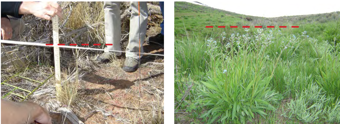
Figure B-3. Grass and forb height measurements. Record natural or “droop” height of grasses and forbs. Note the dashed red reference line.
