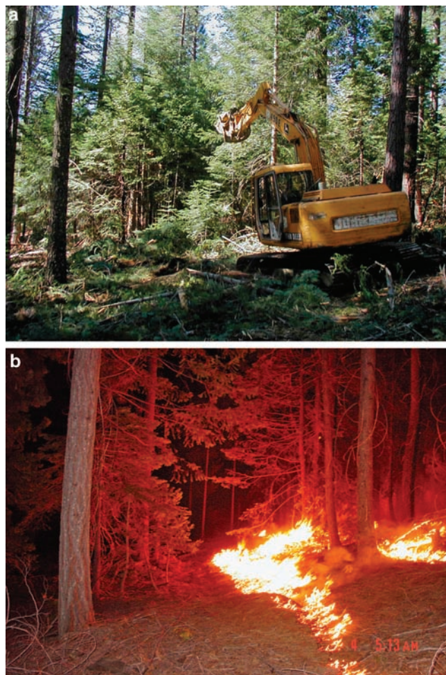
Figure 1. Examples of fire and fire-surrogate treatments applied in order to reduce fire hazards in mixed-conifer forests in the central Sierra Nevada, California. (a) Mechanical fuel treatment using a rotary masticator mounted on an excavator. (b) Prescribed fire at night. Photographs: Jason Moghaddas.
