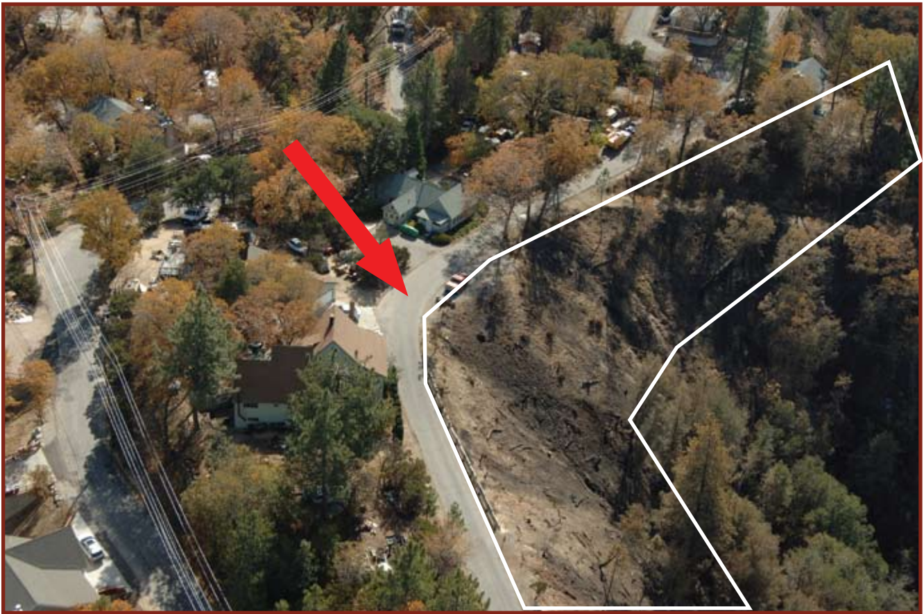
Figure 25. Note location of Edge Cliff Drive (red arrow) and the fuel break below the road (white polygon).
