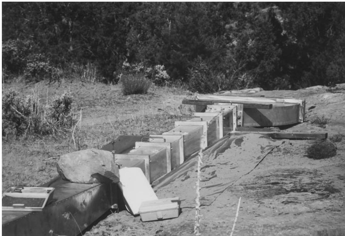
Figure 1. Portable wind tunnel, assembled in the field.
