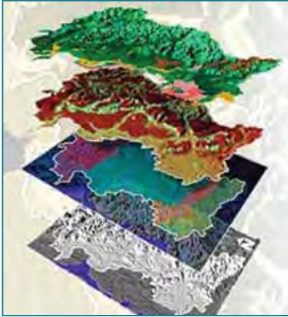
Figure 20—Conceptual image of process-based models that use multiple spatial data sets (e.g., climate, topography, soils, geology, land cover) to estimate the hydrologic behavior of landscapes under varying land-use scenarios, climatic conditions, and disturbance regimes.
