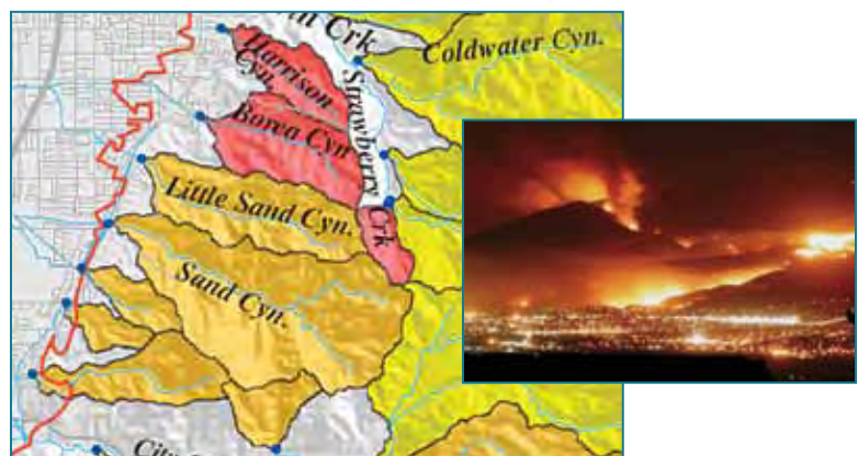
Figure 30—Probability of postfire debris flows associated with the Old Fire in Southern California. Red areas have highest potential, yellow areas the lowest. These risk models were developed by the U.S. Geological Survey and collaborators such as the U.S. Forest Service, Natural Resources Conservation Service, and various state agencies. Improved predictions of postfire effects are needed. Cooperative, interagency efforts offer the greatest potential for meeting critical information needs. Modified from Cannon et al. 2004.
