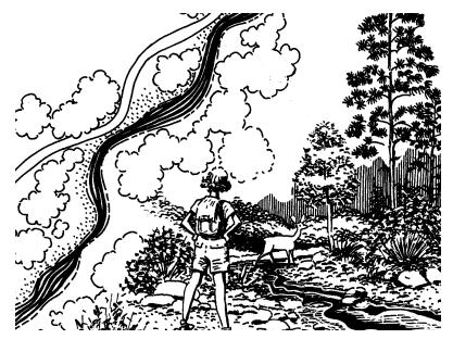
Carefully consider how and where to route a trail through a streamside area. These riparian zones are rich habitat for wildlife. The illustration shows a trail alignment running primarily outside the riparian area, but moving into it at places where wildlife is less likely to be disrupted. (Left: plan view, right: sketch.)
