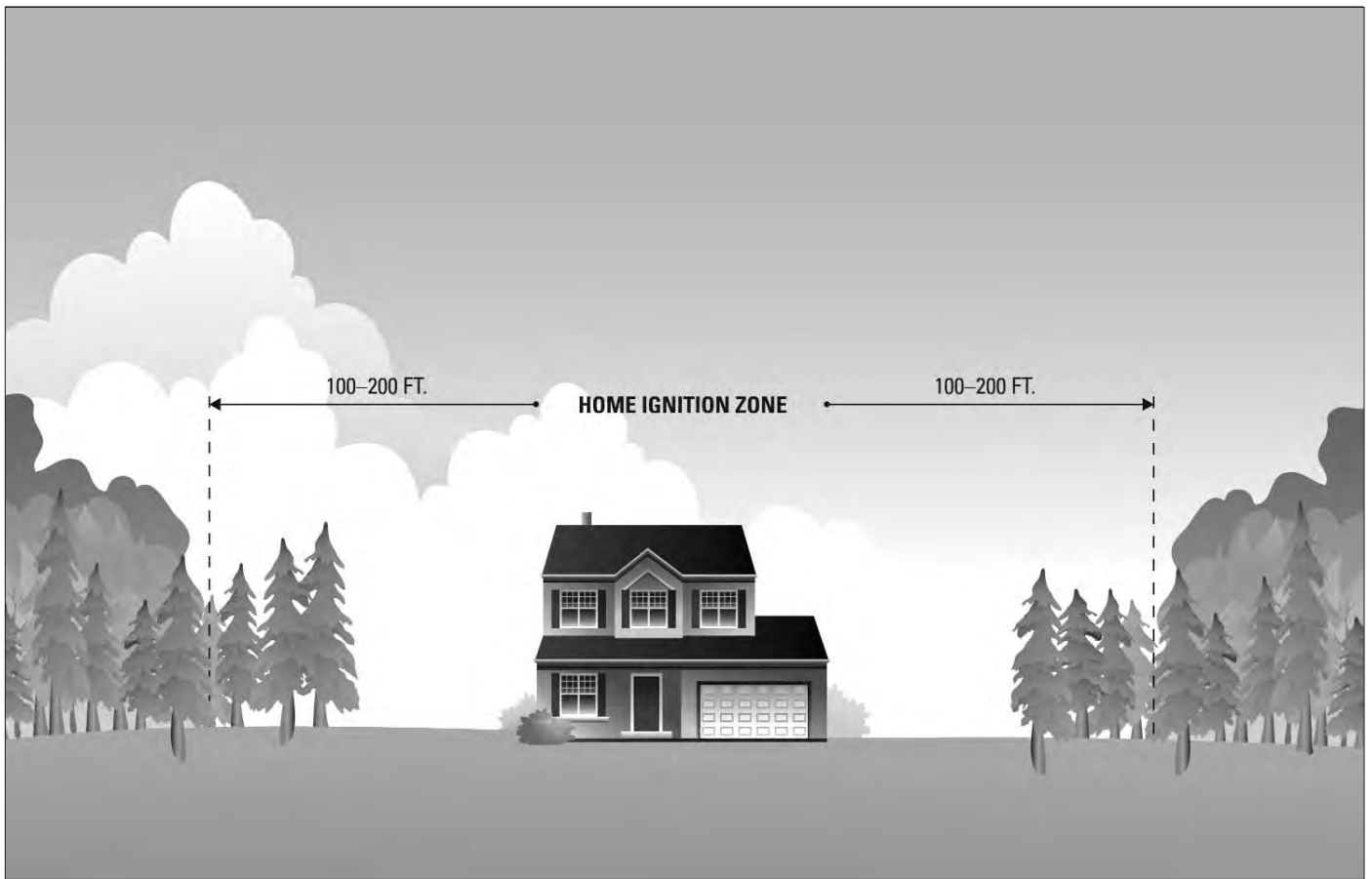
The home ignition zone principally determines a home's ignition potential. The zone includes the home in relation to its surroundings within 100–200 feet of the home.
