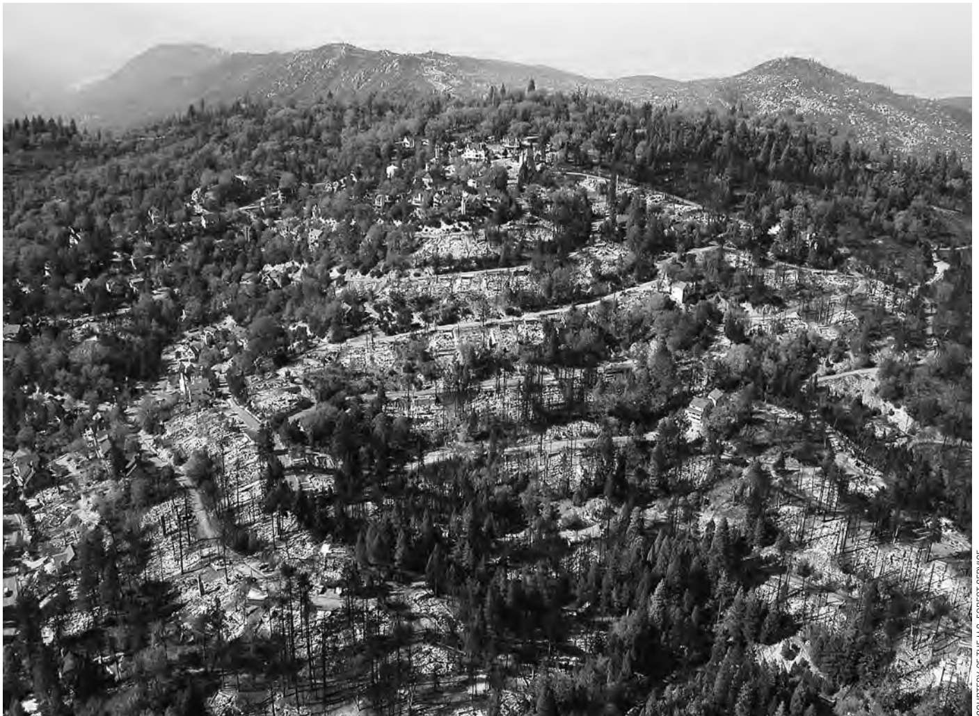
These homes near Lake Arrowhead, California, were destroyed on October 22, 2007, as part of the Grass Valley Fire, and serve as a WUI fire disaster example. Although the homes initially ignited from the wildfire, structures continued to ignite and burn after the wildfire had largely ceased its high-intensity spread.
